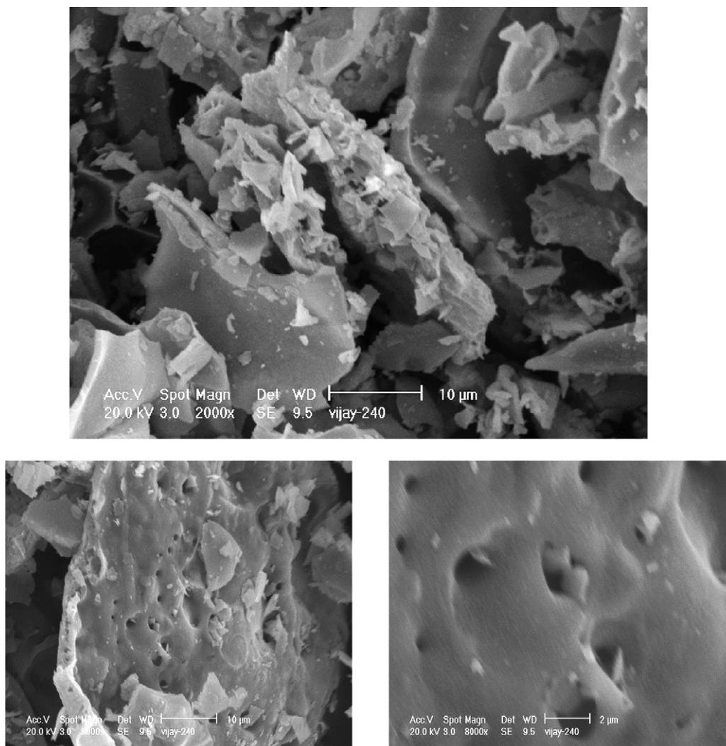
Fig. 3. SEM micrographs of the  $\text{Ba}_{0.99}\text{Cr}_{0.01}\text{Al}_2\text{O}_4$ , at low- and high-magnification.
