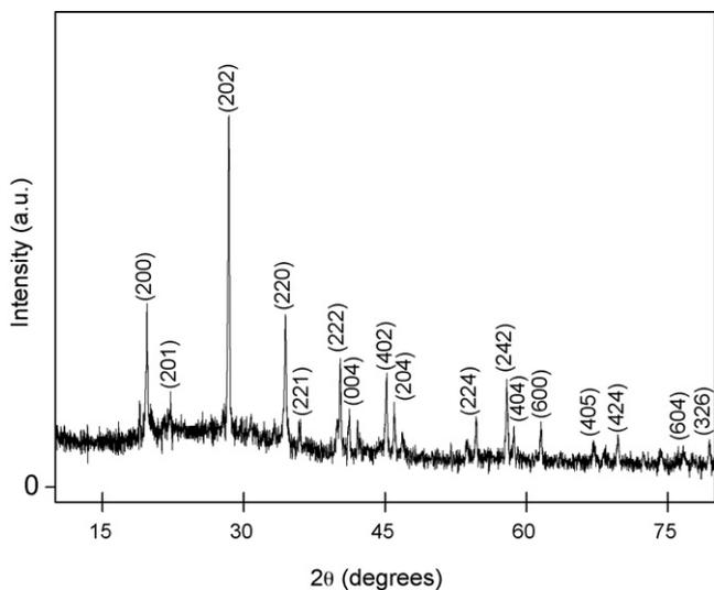
Fig. 1. XRD patterns of  $\text{Ba}_{0.99}\text{Cr}_{0.01}\text{Al}_2\text{O}_4$ .
