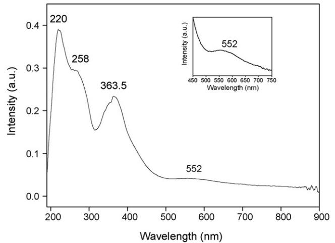
Fig. 5. The UV-vis absorption spectrum of  $\text{Ba}_{0.99}\text{Al}_2\text{O}_4:\text{Cr}_{0.01}$ .
