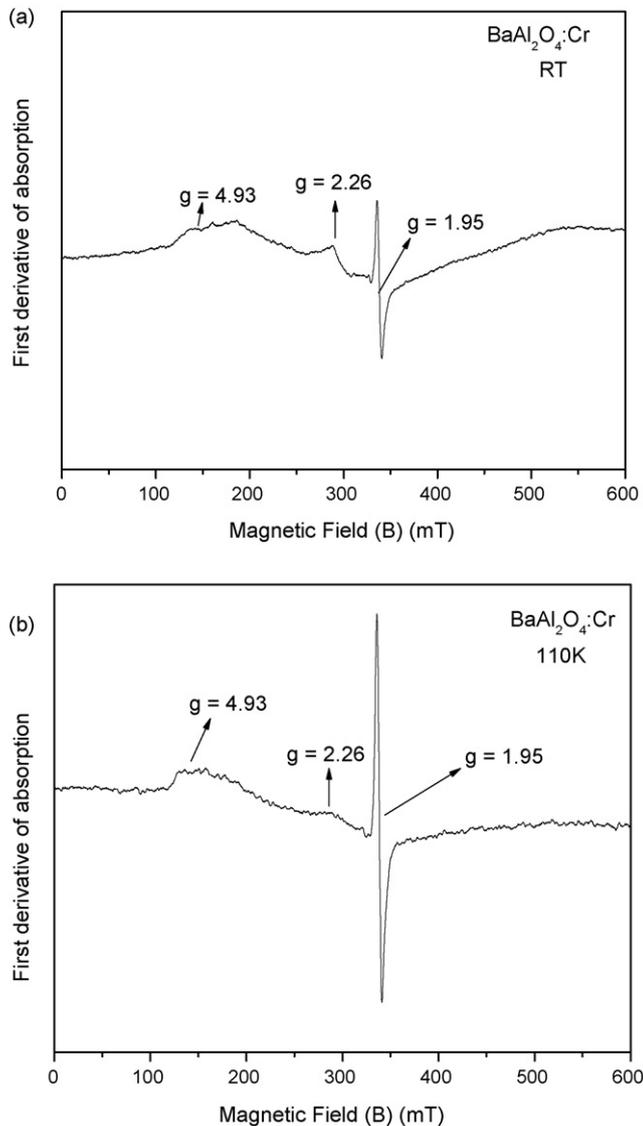
Fig. 4. EPR spectrum of  $\text{Ba}_{0.99}\text{Cr}_{0.01}\text{Al}_2\text{O}_4$  at (a) Room temperature and (b) 110 K.
