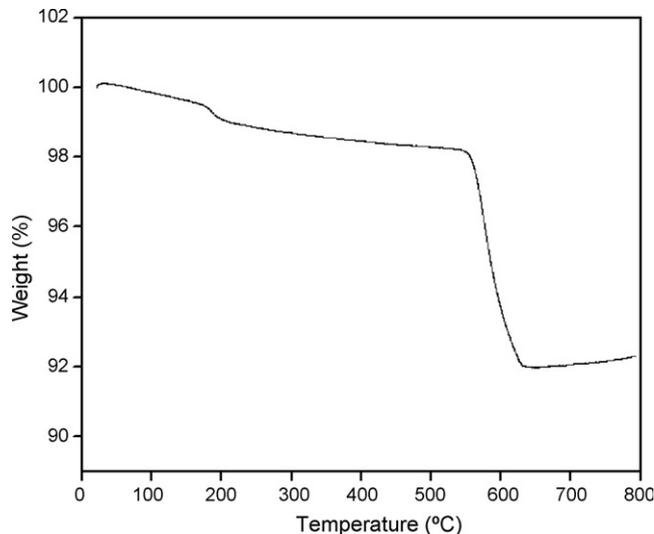
Fig. 2. Thermogravimetric curve of the combustion prepared  $\text{Ba}_{0.99}\text{Cr}_{0.01}\text{Al}_2\text{O}_4$  (heating rate  $10^\circ\text{C min}^{-1}$ ; gas flow-rate:  $40\text{ ml min}^{-1}$ ;  $\text{N}_2$ ).
