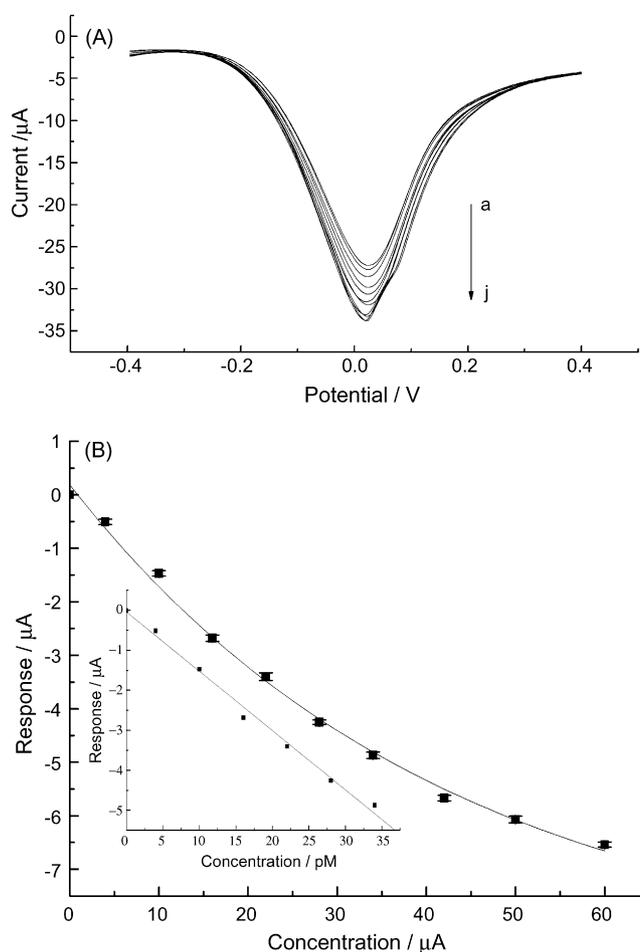
Fig. 7. Differential pulse voltammograms obtained at GOx/AuNPs–AgCl@PANI/GC electrode in 0.1 M phosphate buffer solution (pH 6.0) at 55 °C with glucose of 0 pM (a), 4 pM (b), 10 pM (c), 16 pM (d), 22 pM (e), 28 pM (f), 34 pM (g), 42 pM (h), 50 pM (i), 60 pM (j) (A); relationship between the peak current and the concentration of glucose (B).
