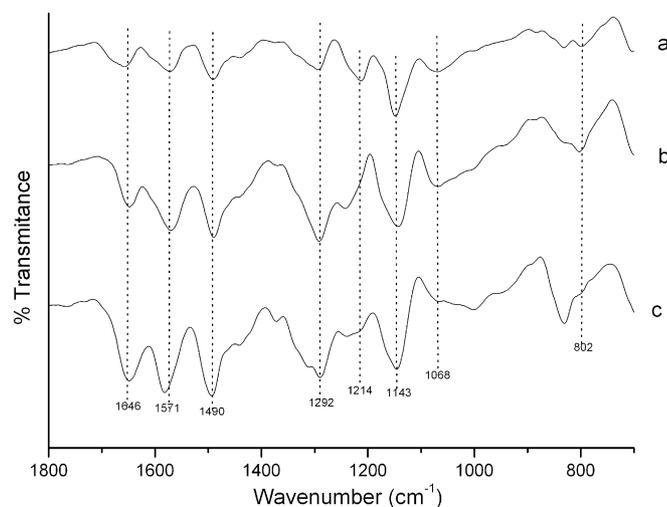
Fig. 3. ATR-FTIR spectra of the films deposited on silicon slides: AgCl@PANI film (a), AuNPs–AgCl@PANI film without (b) and with (c) entrapment of GOx.
