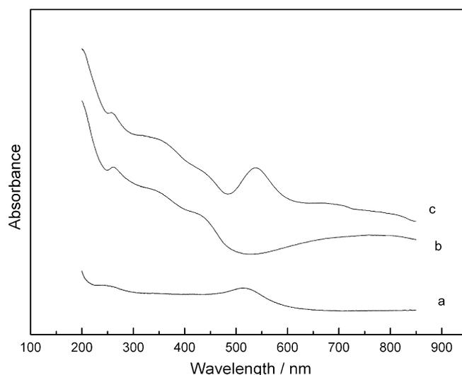
Fig. 2. UV-vis spectra of aqueous dispersion of AuNPs (a), AgCl@PANI (b) and AuNPs–AgCl@PANI (c).
