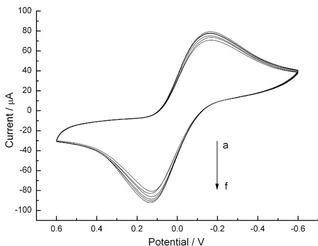
Fig. 5. Cyclic voltammograms obtained at AuNPs–AgCl@PANI modified GC electrode in 0.1 M PBS (pH 6) containing 0 pM (a), 1.0 pM (b), 5.0 pM (c), 10.0 pM (d), 15.0 pM (e), 20.0 pM (f)  $H_2O_2$ .
