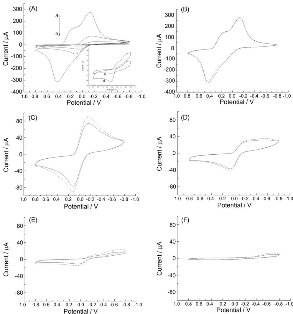
Fig. 4. Cyclic voltammograms obtained at AuNPs–AgCl@PANI modified GC electrode at pH 5 (a), 6 (b), 7 (c), 8 (d), 9 (e) (A); cyclic voltammograms obtained at AuNPs–AgCl@PANI/GC electrode without (real line) and with (dotted line) addition of  $10\text{ }\mu\text{M}$   $\text{H}_2\text{O}_2$  in buffer solutions of different pH values: 5 (B); 6 (C); 7 (D); 8 (E) and 9 (F). (C, D, E and F are of the same scale).
