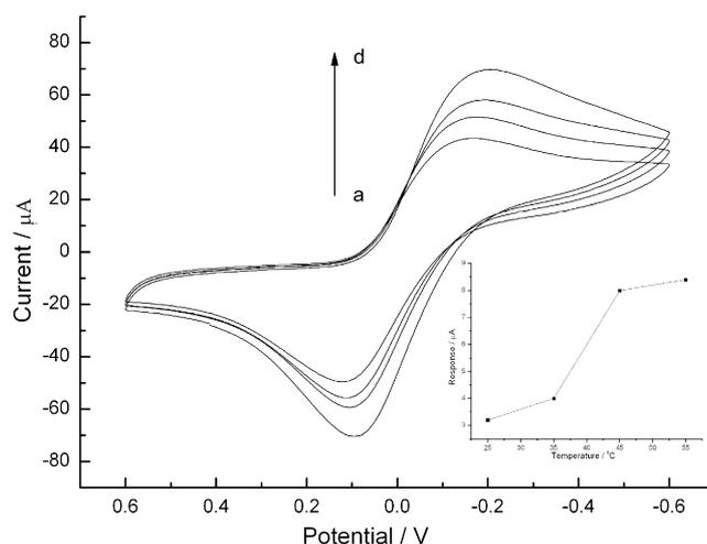
Fig. 6. Cyclic voltammograms obtained at GOx/AuNPs–AgCl@PANI/GC electrode in pH 6.0 PBS without glucose at temperature of  $25^\circ C$  (a),  $35^\circ C$  (b),  $45^\circ C$  (c), and  $55^\circ C$  (d); influence of temperature on the CV response of the biosensor to  $10 \mu M$  glucose in pH 6.0 PBS (insert).
