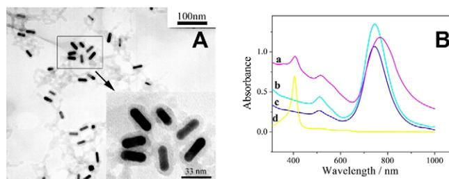
Fig. 1. (A) TEM image of GNRs@SiO<sub>2</sub> composites. (B) UV–visible spectra of (a) Hb–GNRs@SiO<sub>2</sub>, (b) GNRs@SiO<sub>2</sub>, (c) GNRs, and (d) Hb in 0.1 M pH 7.0 PBS.
