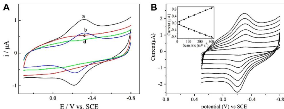
Fig. 2. (A) Cyclic voltammograms of (a) Hb–GNRs@SiO<sub>2</sub>/GCE, (b) Hb–GNRs/GCE, (c) GNRs/GCE, and (d) GNRs@SiO<sub>2</sub>/GCE in 0.1 M pH 7.0 PBS at 0.1 V s<sup>-1</sup>. (B) Cyclic voltammograms of Hb–GNRs@SiO<sub>2</sub>-modified GCE at scan rate of 20, 60, 100, 150, 200, 250, and 300 mV s<sup>-1</sup> in 0.1 M pH 7.0 PBS, respectively and (inset) plots of peak currents vs. scan rates.
