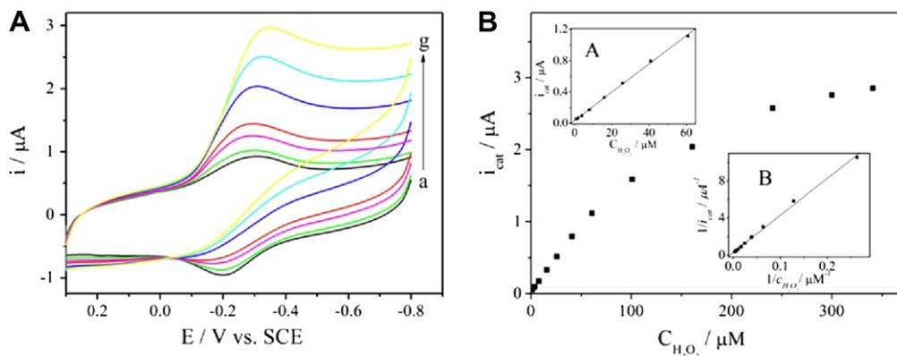
Fig. 3. (A) Cyclic voltammograms of the Hb-GNRs@SiO<sub>2</sub>/GCE at scan rate of 0.1 V s<sup>-1</sup> in 0.1 M pH 7.0 PBS solution with (a) 0, (b) 3.8, (c) 15.8, (d) 25.8, (e) 60.8, (f) 100.8 and (g) 160.8 μM H<sub>2</sub>O<sub>2</sub>. (B) Plots of the electrocatalytic current ( $I_{\text{cat}}$ ) vs. H<sub>2</sub>O<sub>2</sub> concentration. Inset: Linear plots of  $I_{\text{cat}}$  vs. H<sub>2</sub>O<sub>2</sub> concentration (A) and the Lineweaver–Burk plot (B).
