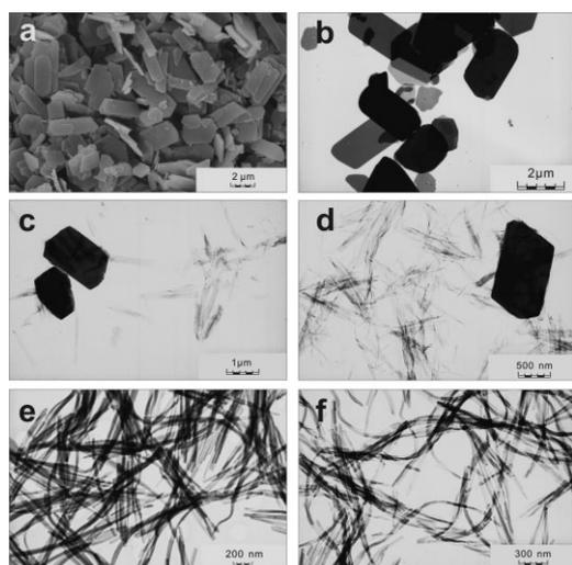
**Figure 3.** a) SEM image of the product synthesized at a CdCl<sub>2</sub>/q ratio of 1:5. TEM images of the products synthesized at CdCl<sub>2</sub>/q ratios of b) 1:5, c) 1:3, d) 1:1, e) 3:1, and f) 5:1. The reaction time was 50 min.
