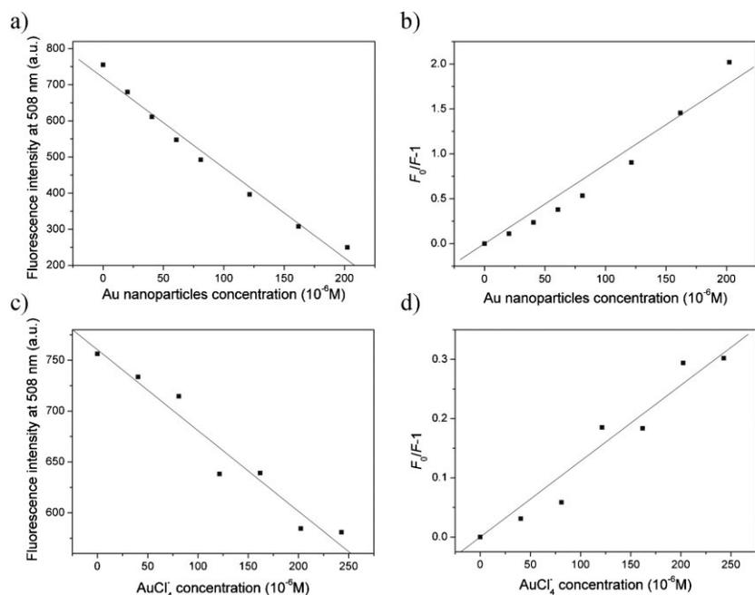
**Figure 8.** The fluorescence quenching of CdqCl nanowires by Au nanoparticles: a) the fluorescence intensity at 508 nm versus Au nanoparticle concentration, b) S–V plot. The fluorescence quenching of CdqCl nanowires by AuCl<sub>4</sub><sup>−</sup> nanoparticles: c) the fluorescence intensity at 508 nm versus AuCl<sub>4</sub><sup>−</sup> concentration, d) S–V plot.
