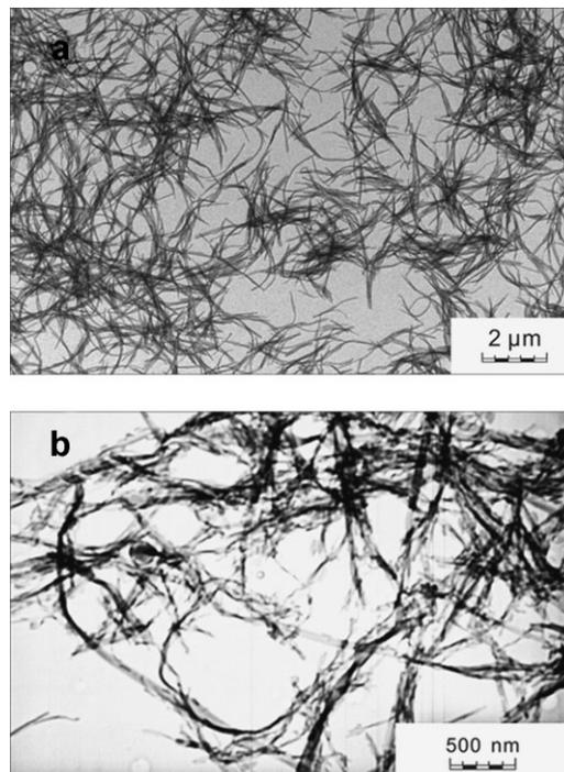
Figure 5. TEM images of the  $\text{CdqCl}$  nanowires obtained with a) ultrasound irradiation and b) electromagnetic stirring ( $\text{CdCl}_2/\text{q} = 3:1$ ).
