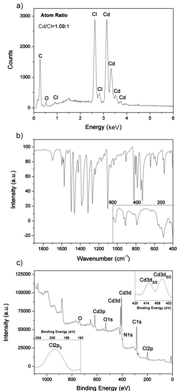
**Figure 1.** Spectral measurements of CdqCl nanowires: a) EDX spectrum, b) infrared (IR) spectra, inset: Far-IR spectrum, c) X-ray photoelectron spectroscopy (XPS) analysis, inset: high-resolution XPS in the Cd  $3d$  (top-right) and Cl  $2p$  (bottom-left) regions.
