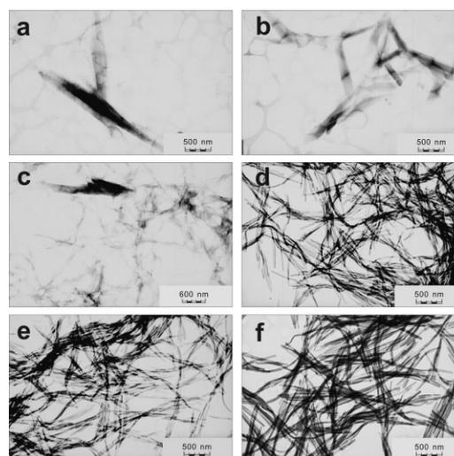
**Figure 4.** TEM images of the samples obtained at different reaction times: a) 2, b) 12, c) 20, d) 30, e) 50, and f) 120 min.
