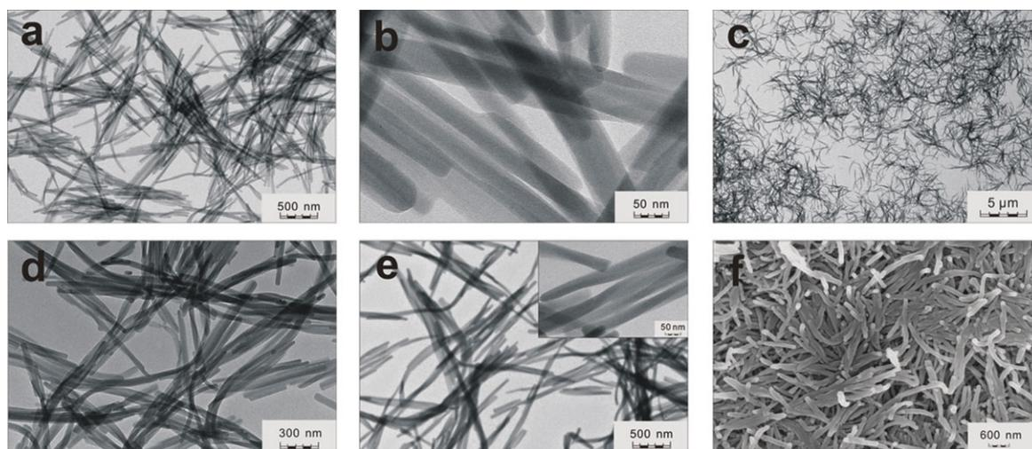
**Figure 2.** TEM images of CdqCl nanowires synthesized at CdCl<sub>2</sub>/q ratios of a,b) 3:1, c,d) 5:1, e) 10:1. f) SEM image of CdqCl nanowires synthesized at a CdCl<sub>2</sub>/q ratio of 3:1. The reaction times were a–e) 50 min and f) 120 min.
