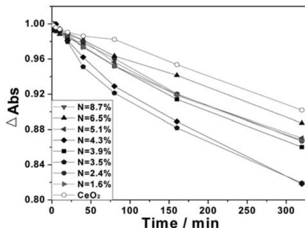
Fig. 5 Methylene blue photodecomposition catalyzed by  $\text{CeO}_{2-x}\text{N}_x$  nanoparticles upon photoexcitation with wavelength  $> 500$  nm.
