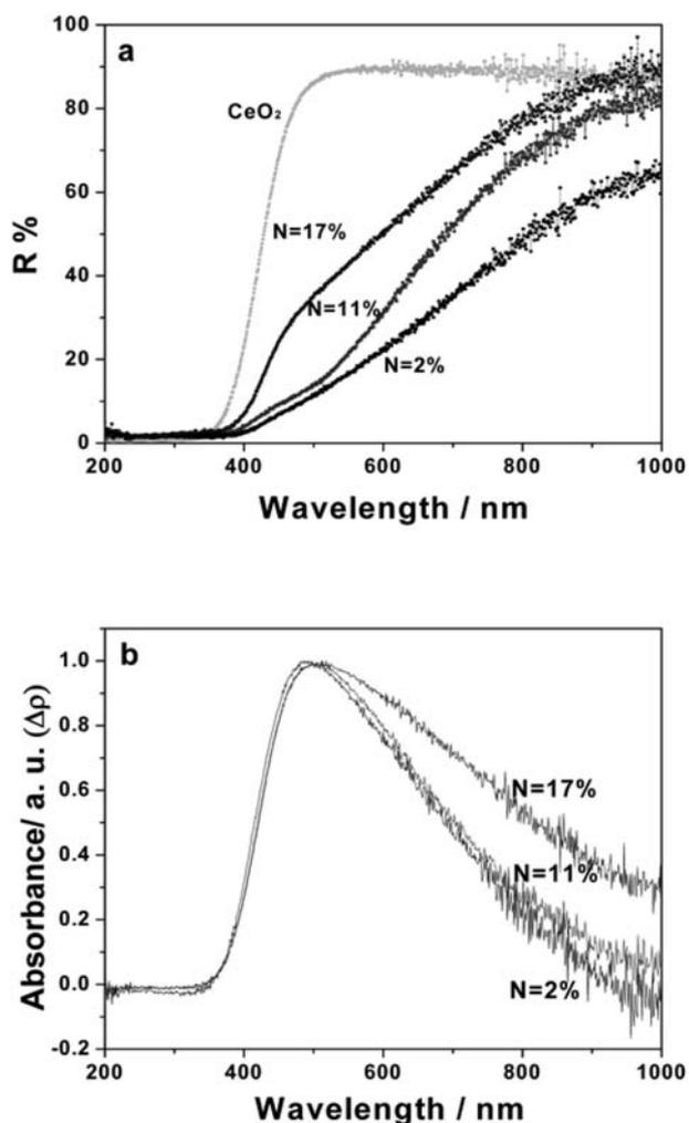
Fig. 3 UV-Vis diffuse reflectance spectra (DRS) (a) and difference DRS spectra ( $\Delta\rho$ ) (b) of CeO<sub>2–x</sub>N<sub>x</sub> nanoparticle powders.
