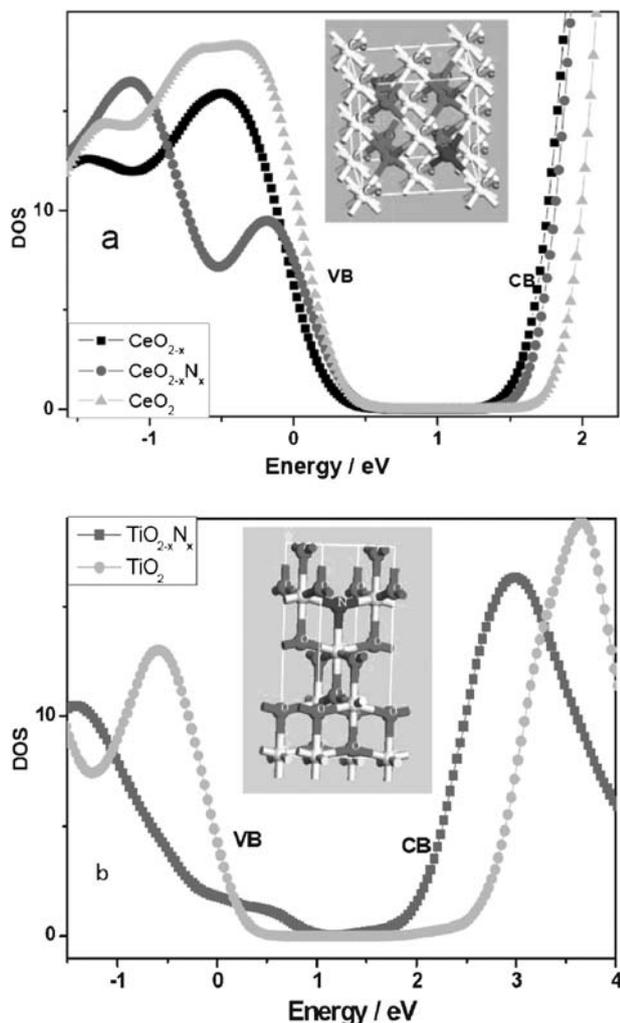
Fig. 4 DFT calculations of the densities of states of fluorite-type  $\text{CeO}_2$  with substituted oxygen sites as indicated in the inset.
