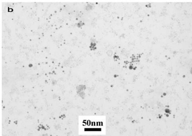
**Fig. 1** (a) XRD patterns for  $\text{CeO}_2$  and N-doped  $\text{CeO}_2$  at different sintered temperatures. (b) TEM image of N-doped  $\text{CeO}_2$ .
