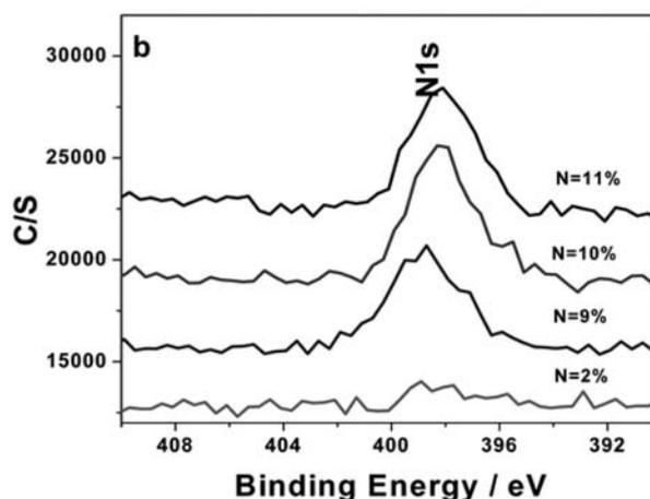
**Fig. 2** The full scale XPS spectra of  $\text{CeO}_{2-x}\text{N}_x$  nanoparticles with different N-doping levels. Fig. 2b contains the enlarged N 1s regions of the corresponding full scale XPS spectra.
