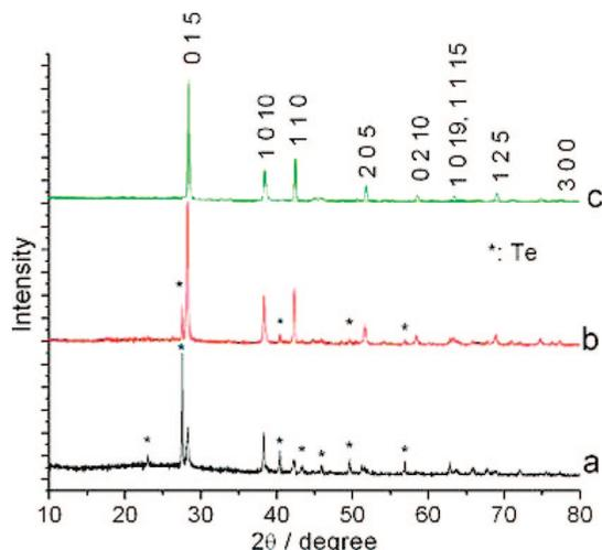
**Figure 1.** XRD patterns of the products obtained after (a) 10, (b) 25, and (c) 45 min of microwave-assisted reaction.
