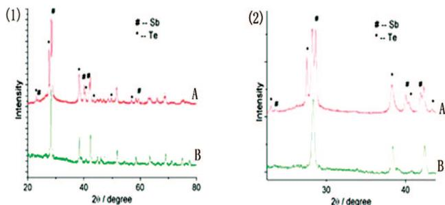
**Figure 4.** XRD patterns (in different magnification for (1) and (2)) of products obtained after reacted for (A) 1 h and (B) 2 h, with the addition of 0.5 g of PVP. The XRD peaks marked with “#” were in good agreement with those reported in the literature (JCPDS File No. 71–1173, hexagonal Sb). The XRD peaks marked with “\*” could be indexed to hexagonal Te (JCPDS File No. 36–1452).
