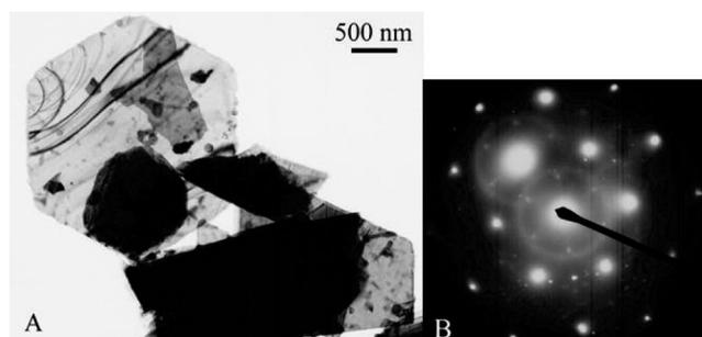
**Figure 3.** (A) TEM image and (B) SAED pattern of as-prepared Sb<sub>2</sub>Te<sub>3</sub>.
