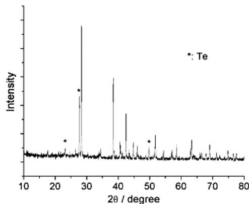
**Figure 2.** XRD pattern of Sb<sub>2</sub>Te<sub>3</sub> obtained after 48 h of solvothermal reaction.
