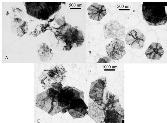
**Figure 5.** TEM images of  $\text{Sb}_2\text{Te}_3$  prepared with the addition of various amounts of PVP and after various reaction time: (A) 0.1 g of PVP, 2 h; (B) 0.5 g of PVP, 2 h; (C) 0.1 g of PVP, 3 h.
