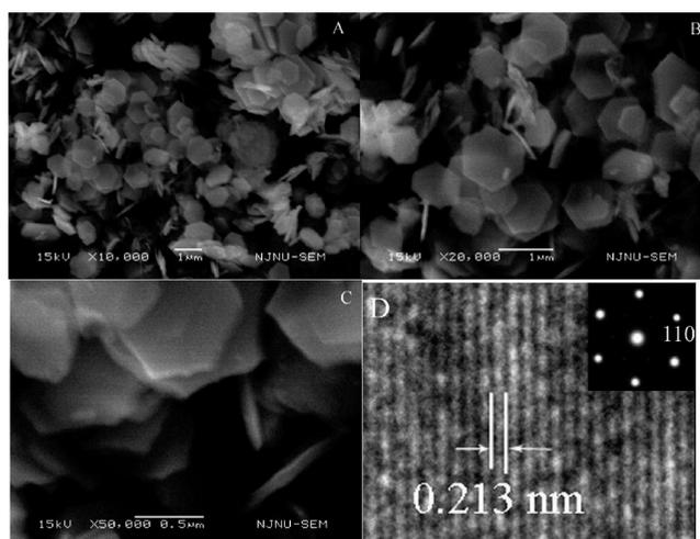
**Figure 6.** (A–C) SEM images in various magnifications of  $\text{Sb}_2\text{Te}_3$  prepared with the addition of 0.5 g of PVP and after 2 h of reaction; (D) HRTEM image and SAED pattern (the insert) of the same sample.
