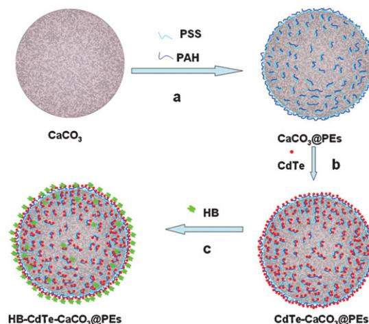
**Scheme 1.** Schematic illustration of the fabrication process of the HB-CdTe-CaCO<sub>3</sub>@PEs 3D architecture. a) CaCO<sub>3</sub> microspheres were firstly coated with polyelectrolyte layers to produce CaCO<sub>3</sub>@PEs microspheres. b) The polyelectrolyte-protected spheres were then used for the loading of CdTe quantum dots to fabricate the CdTe-CaCO<sub>3</sub>@PEs hybrid material. c) In the final step, the hybrid material was used for the loading of hemoglobin (HB).
