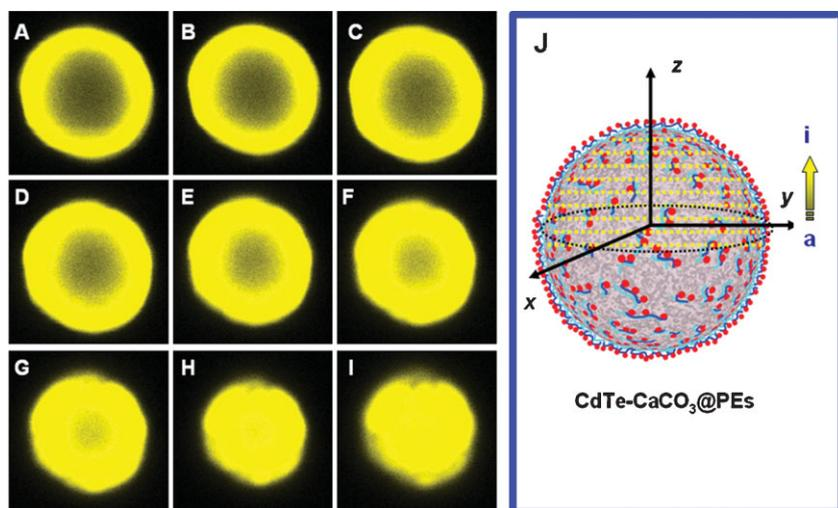
**Figure 6.** A–I) A series of confocal images of CdTe-CaCO<sub>3</sub>@PEs microsphere taken sequentially along the z-axis from the center of the CdTe-CaCO<sub>3</sub>@PEs sphere to the top. J) A schematic illustration of how the Z-series is taken. The yellow dashed lines (a–i) represent the levels perpendicular to the optical axis (the z-axis) within the microsphere.
