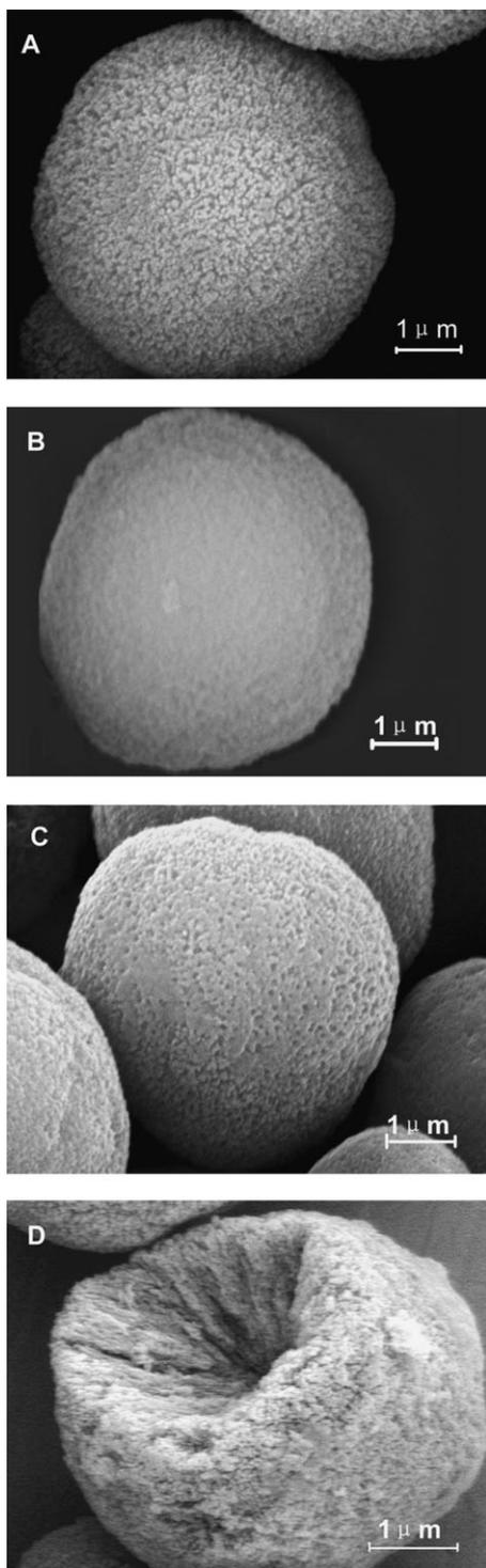
**Figure 3.** SEM images of A) CaCO<sub>3</sub>@PEs; B) CdTe-CaCO<sub>3</sub>@PEs; C) HB-CdTe-CaCO<sub>3</sub>@PEs spheres; and D) a broken CdTe-CaCO<sub>3</sub>@PEs sphere at higher magnification.
