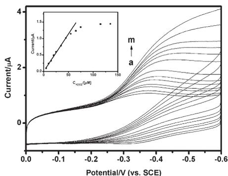
**Figure 11.** Cyclic voltammograms of HB-CdTe-CaCO<sub>3</sub>@PEs/PVA-modified GCEs in 0.1 M PBS at pH = 7.0 in the presence of: a) 0, b) 5, c) 10, d) 15, e) 20, f) 25, g) 35, h) 45, i) 55, j) 65, k) 75, l) 135, and m) 205 µM H<sub>2</sub>O<sub>2</sub> at a scan rate of 200 mV s<sup>-1</sup>. The insert shows the calibration curve.
