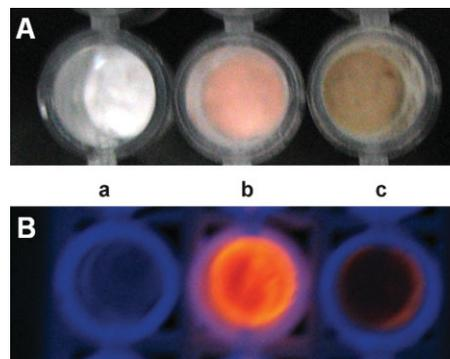
**Figure 8.** A) Images of a) CaCO<sub>3</sub>@PEs, b) CdTe-CaCO<sub>3</sub>@PEs and c) HB-CdTe-CaCO<sub>3</sub>@PEs under ambient light. B) Images of a) CaCO<sub>3</sub>@PEs, b) CdTe-CaCO<sub>3</sub>@PEs, and c) HB-CdTe-CaCO<sub>3</sub>@PEs under 260 nm UV illumination.
