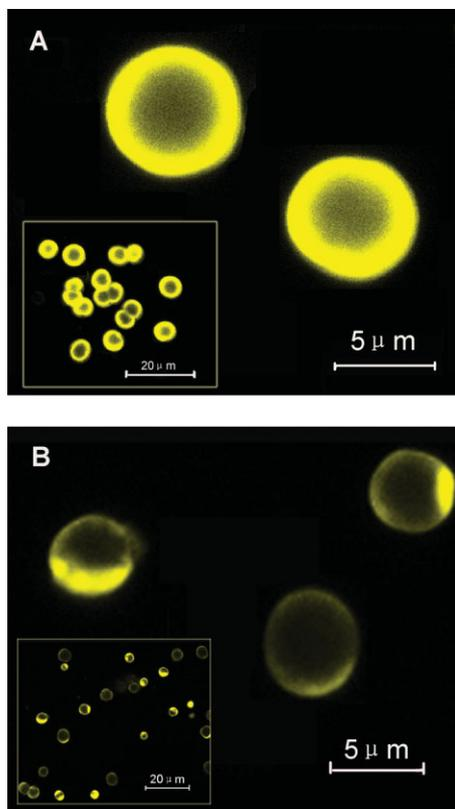
**Figure 4.** Confocal images of A) CdTe-CaCO<sub>3</sub> microspheres and B) CdTe-CaCO<sub>3</sub>@PEs microspheres. The inserts show the overviews of the spheres.
