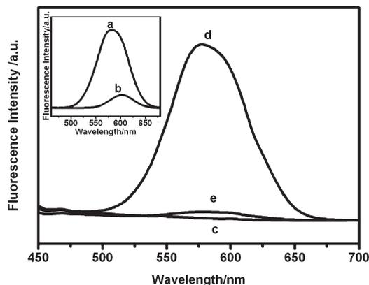
**Figure 2.** Fluorescence spectra of a) the as-prepared CdTe; b) the supernatant after the absorption of CdTe QDs onto the CaCO<sub>3</sub>@PEs spheres; c) CaCO<sub>3</sub>@PEs spheres; d) CdTe-CaCO<sub>3</sub>@PEs spheres; and e) HB-CdTe-CaCO<sub>3</sub>@PEs spheres.
