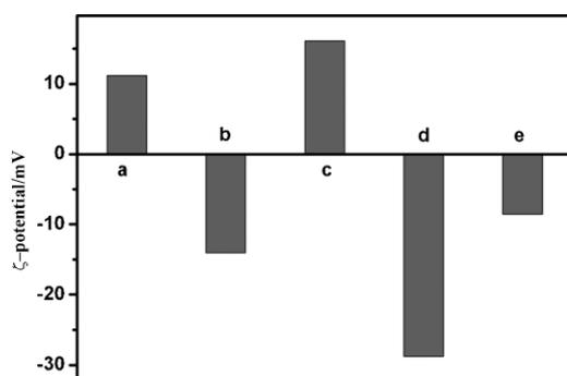
**Figure 1.** The values of the  $\zeta$ -potentials during the whole assembly process. The bars represent a) CaCO<sub>3</sub>; b) CaCO<sub>3</sub>/PSS; c) CaCO<sub>3</sub>@PEs; d) CdTe-CaCO<sub>3</sub>@PEs; and e) HB-CdTe-CaCO<sub>3</sub>@PEs microspheres.
