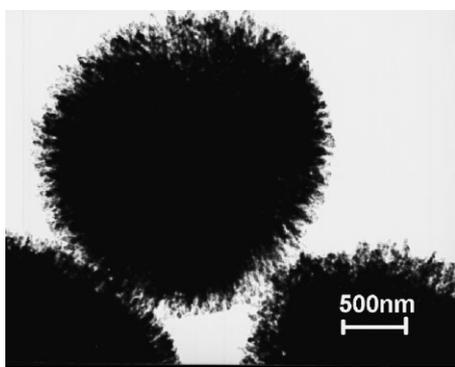
**Figure 5.** TEM image of CdTe-CaCO<sub>3</sub>@PEs microspheres, illustrating the presence of CdTe QDs.
