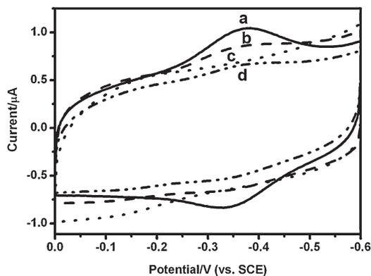
**Figure 9.** Cyclic voltammograms of a) HB-CdTe-CaCO<sub>3</sub>@PEs/PVA, b) HB-CaCO<sub>3</sub>@PEs/PVA, c) CdTe-CaCO<sub>3</sub>@PEs/PVA, and d) HB-CdTe-MPS@PAH/PVA-modified glassy carbon electrode (GCE) in 0.1 M PBS at pH = 7.0 and a scan rate of 200 mV s<sup>-1</sup>.
