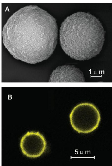
**Figure 7.** A) SEM image of conventional mesoporous silica (MPS) spheres used in comparison experiment. B) Confocal image of CdTe-MPS-PAH spheres.
