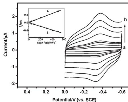
**Figure 10.** Cyclic voltammograms of HB-CdTe-CaCO<sub>3</sub>@PEs/PVA-modified GCE in 0.1 M PBS at pH = 7.0 and at different scan rates. The scan rate from the inner to the outer curves were: a) 20, b) 50, c) 80, d) 100, e) 200, f) 300, g) 400, and h) 500 mV s<sup>-1</sup>. The insert shows the plot of A) the anodic and B) the cathodic peak currents vs. scan rate.
