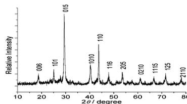
**Figure 3.** XRD pattern of the product obtained after reacted in alkaline solution (containing 1 g of KOH) for 24 h in the synthesis of  $Bi_2Se_3$ .
