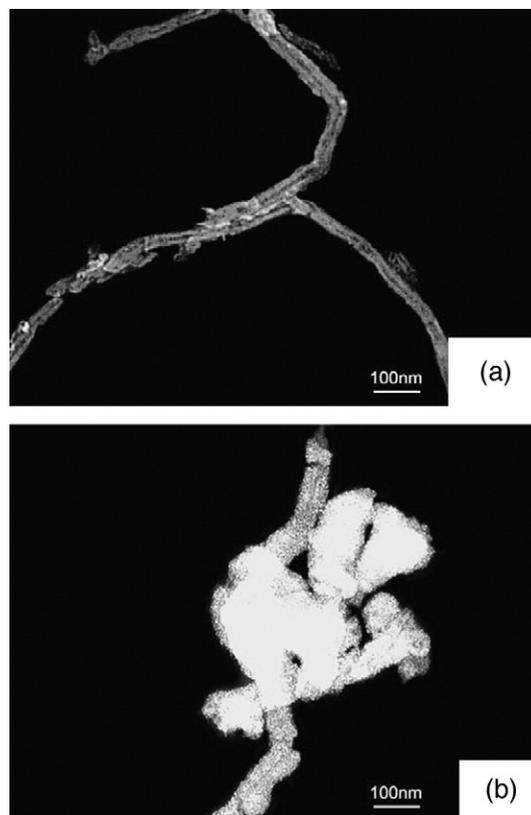
Fig. 1. TEM images of A-MWCNTs (a) and TiO<sub>2</sub>/MWCNTs composites (b).
