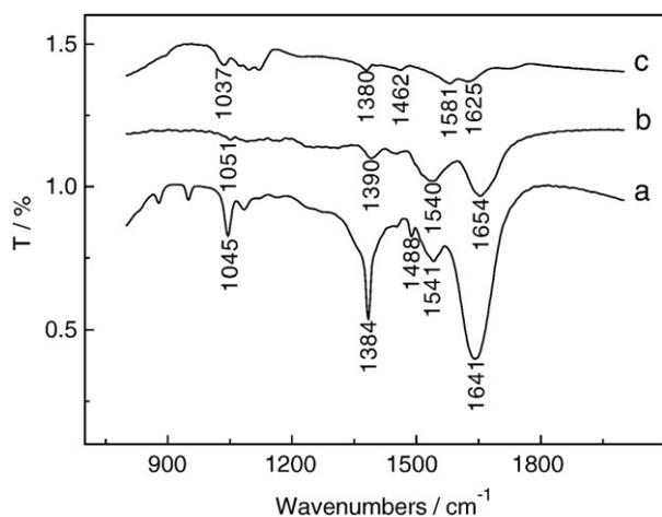
Fig. 3. FTIR spectra of Mb–TiO<sub>2</sub>/MWCNTs (a), free Mb (b), TiO<sub>2</sub>/MWCNTs (c) film.
