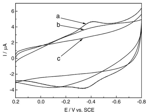
Fig. 4. CVs obtained with Mb–TiO<sub>2</sub>/MWCNTs film modified GC electrodes (a), TiO<sub>2</sub>/MWCNTs film modified GC electrodes (b) and bare GC electrodes (c) in 0.1 M PBS (pH 7.0) at 100 mV/s.
