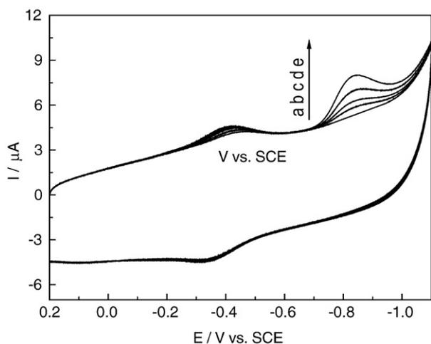
**Fig. 10.** CVs at 100 mV/s in pH 7.0 PBS for Mb-TiO<sub>2</sub>/MWCNTs modified GC electrode in PBS containing no NO (a), as (a) in the presence 0.1, 0.2, 0.4 and 0.8 mM of NO (b, c, d and d).
