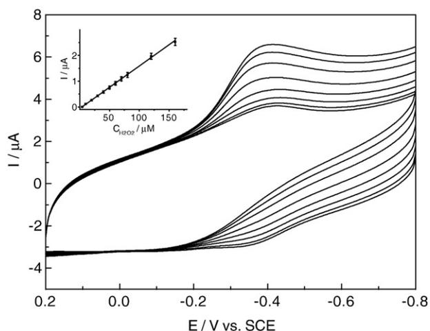
**Fig. 8.** CVs of Mb-TiO<sub>2</sub>/MWCNTs GC electrode in the presence of different concentration of H<sub>2</sub>O<sub>2</sub> in PBS (pH 7.0) at 100 mV/s, from inner to outer 0, 4, 10, 20, 40, 80, 120 and 160 μM. Inset: the catalytic response vs. hydrogen peroxide concentrations.
