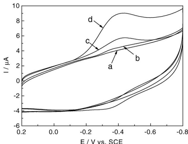
Fig. 7. CVs at 100 mV/s in pH 7.0 PBS for TiO<sub>2</sub>/MWCNTs GC electrodes in PBS containing no H<sub>2</sub>O<sub>2</sub> (a), as (a) in the presence 0.2 mM of H<sub>2</sub>O<sub>2</sub> (b), (c) and (d) as (a) and (b) for Mb–TiO<sub>2</sub>/MWCNTs modified GC electrodes.
