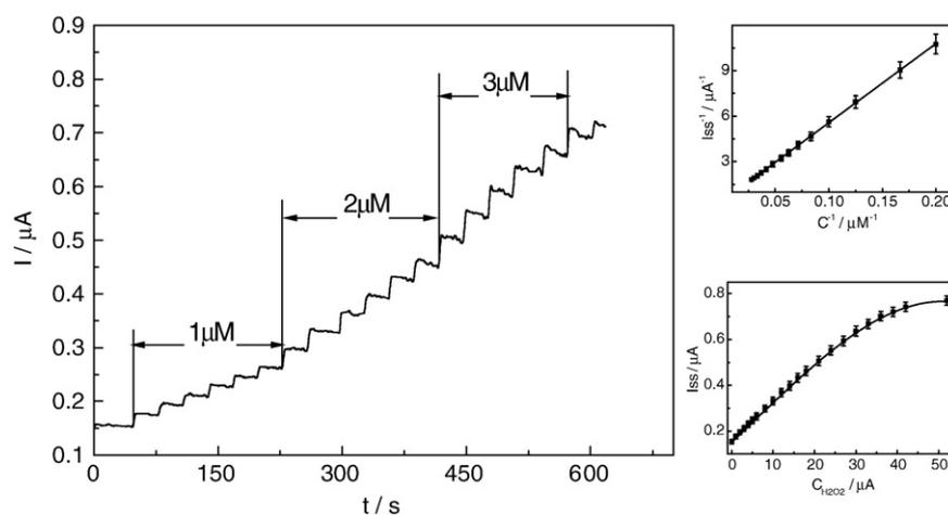
**Fig. 9.** Amperometric response of Mb-TiO<sub>2</sub>/MWCNTs GC electrode with successive addition of H<sub>2</sub>O<sub>2</sub> to the 0.1 M pH 7.0 PBS under stirring. The applied potential was -0.4 V.
