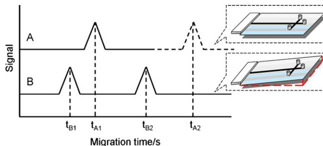
Fig. 1. Schematic electrophoretograms and diagrams of non-tilting microchip (A) and tilting microchip (B), and define them as pattern A and pattern B, respectively.
