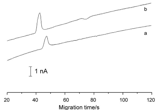
**Fig. 3.** Electrophoretograms for low EOF measurement with sampling zone detection in BSA coated PDMS channels. (a) In non-tilting microchip and (b) in tilting microchip with 15° tilted angle. Sample, 30 mM PB; running buffer, 20 mM PB + 0.1 mM DHBA; pH 6.98. Experimental parameters: sampling voltage, 600 V; sampling time, 2 s; separation voltage, 600 V; detection potential, +1.4 V.
