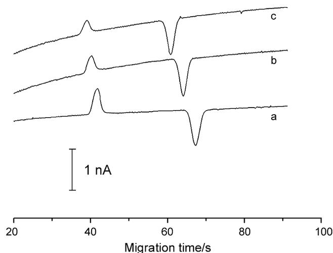
**Fig. 2.** Electrophoretograms illustrating the effect of different tilted angle on liquid flow in native PDMS channel. (a) 0° tilted angle, (b) 7° tilted angle and (c) 15° tilted angle. Sample, 30 mM PB; running buffer, 20 mM PB + 0.1 mM DHBA; pH 6.98. Experimental parameters: sampling voltage, 600 V; sampling time, 2 s; separation voltage, 600 V; detection potential, +1.4 V.
