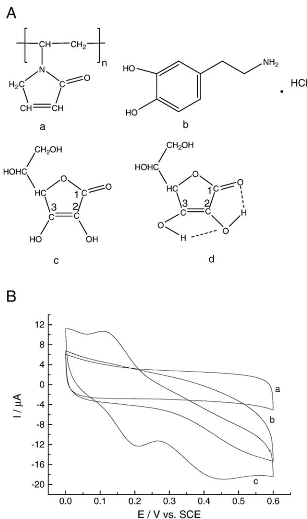
Fig. 5. Molecular structures of PVP (a), dopamine (b), ascorbic acid (c) and intramolecular hydrogen bonding of ascorbic acid (d) (A). Cyclic voltammograms of PVP modified GC electrode. Curve (a): pH 7.0 phosphate buffer (0.1 M); Curve (b): (a) +1 mM ascorbic acid; Curve (c): (a) +1 mM dopamine (Scan rate: 0.1 V s<sup>-1</sup>) (B).
