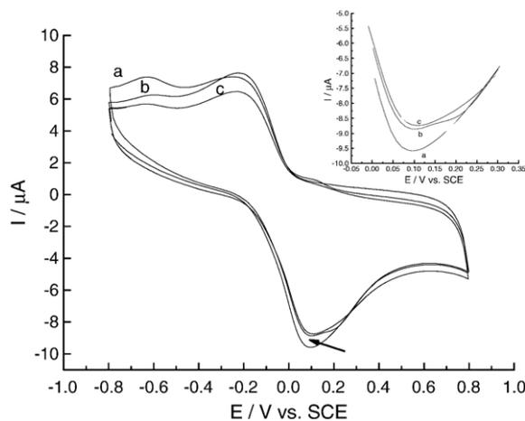
Fig. 3. Cyclic voltammograms of AgCl@PANI/GC electrode. Curve (a): pH 7.0 phosphate buffer (0.1 M); Curve (b): (a) + 1 mM dopamine; Curve (c): (a) + 1 mM ascorbic acid (Scan rate:  $0.1 \text{ V s}^{-1}$ ). The insert shows the enlarged view of the region indicated by the arrow.
