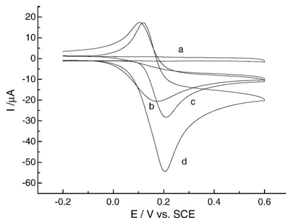
Fig. 2. Cyclic voltammograms of bare GC electrode. Curve (a): pH 7.0 phosphate buffer (0.1 M); Curve (b): (a) + 1 mM ascorbic acid; Curve (c): (a) + 1 mM dopamine; Curve (d): (a) + a mixture of 1 mM dopamine and 1 mM ascorbic acid. Scan rate:  $0.1 \text{ V s}^{-1}$ .
