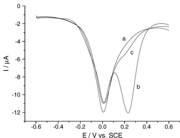
Fig. 4. Square-wave voltammograms of AgCl@PANI/GC electrode. Curve (a): pH 7.0 phosphate buffer; Curve (b): (a) +0.1 mM dopamine; Curve (c): (a) +1 mM ascorbic acid.
