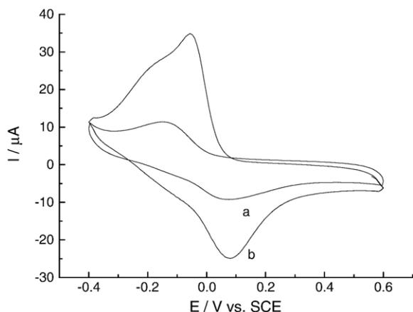
Fig. 6. Cyclic voltammograms of AgCl@PANI/GC electrode (a) and Nafion–AgCl@PANI/GC electrode (b) in pH 7.0 phosphate buffer (0.1 M). Scan rate:  $0.1 \text{ V s}^{-1}$ .
