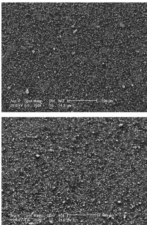
Fig. 1. SEM images of AgCl@PANI nanocomposite (up) and Nafion coated AgCl@PANI nanocomposite films (down) on silicon wafers.
