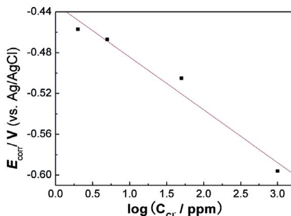
Fig. 6. Dependence of the corrosion potential ( $E_{\text{corr}}$ ) on  $\log C_{\text{Cl}^-}$  for aluminum tabs.
