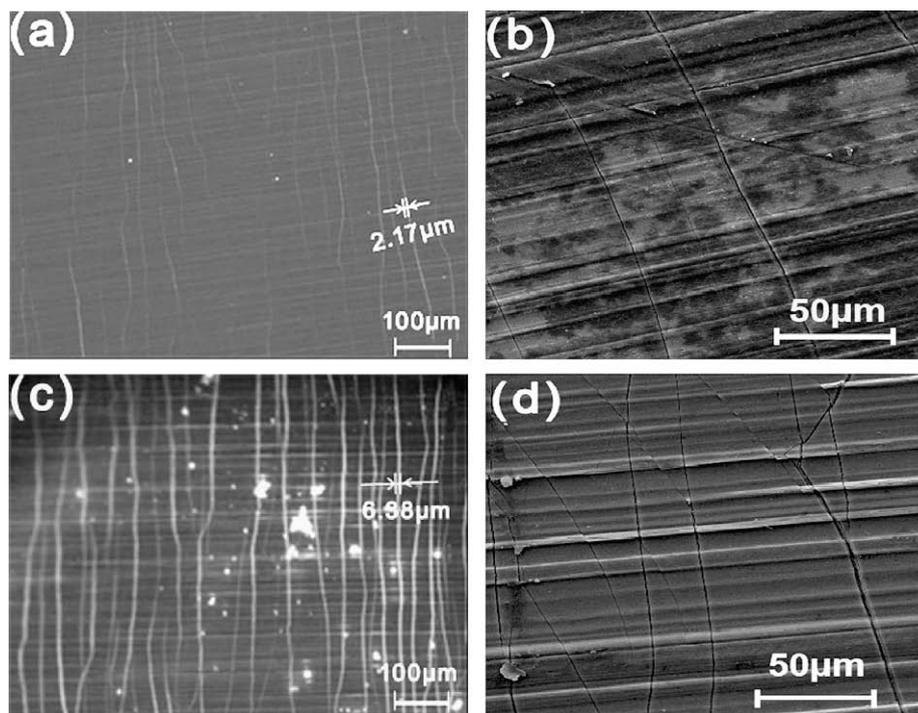
**Fig. 4.** OM images (a and c) and SEM images (b and d) of aluminum tabs anodized potentiostatically after the anodic polarization in the ethyleneglycol–borate solution with chloride ions of 0 ppm(a and b) and 2 ppm (c and d).
