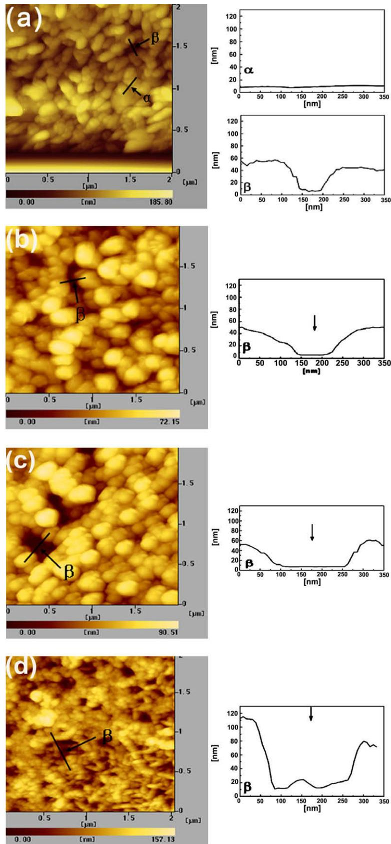
**Fig. 2.** AFM images ( $2 \times 2 \mu\text{m}^2$ ) of aluminum tabs anodized potentiostatically in the solution with chloride ions of (a) 0 ppm, (b) 2 ppm, (c) 50 ppm and (d) 1000 ppm. Examples of the different types of pits are marked with arrows in the images and illustrated by cross-sections.
