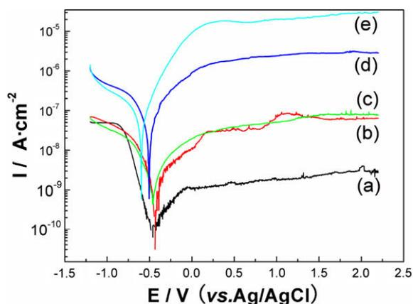
Fig. 5. Polarization curves of the aluminum tabs in ethyleneglycol-borate solution with chloride ions: (a) 0 ppm, (b) 2 ppm, (c) 5 ppm, (d) 50 ppm and (e) 1000 ppm.
