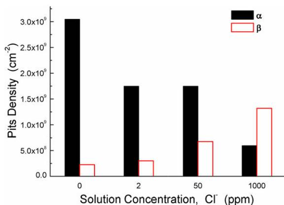
**Fig. 3.** Dependence of the pits density on  $\text{Cl}^-$  concentration in ethyleneglycol–borate solution.
