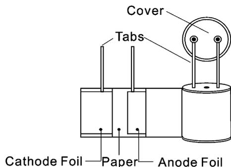
Fig. 1. Schematic of the aluminum (Al) electrolytic capacitor.
