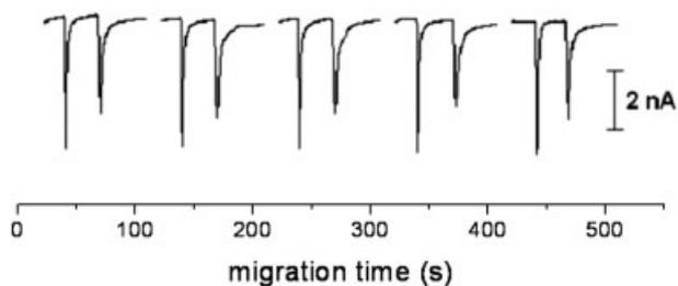
**Figure 6.** Electropherogram of a sequence separation of 500  $\mu\text{M}$  dopamine and catechol with 17° tilted microchip hydrostatic pressure injection, periodical injection time is 40 s. Detection potential: +1.4 V.
