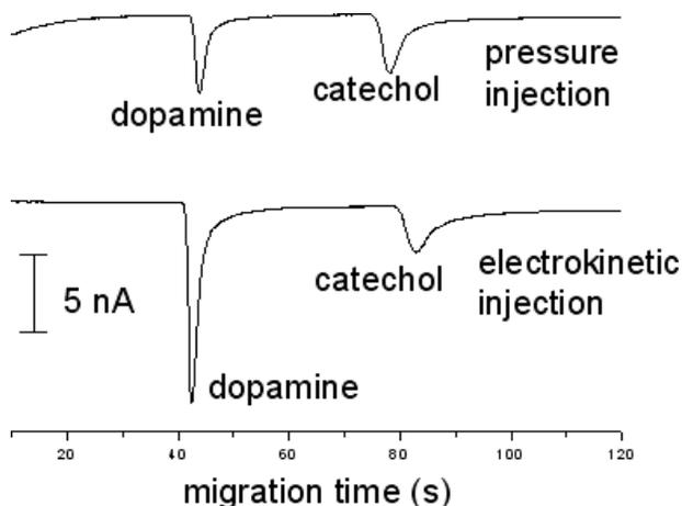
**Figure 7.** Electropherograms for the separation of 500  $\mu\text{M}$  dopamine and catechol with different injection mode. Separation voltage: 800 V, detection voltage: +1.4 V. (A) Tilted microchip hydrostatic pressure injection with 17° tilted angle, injection duration: 40 s. (B) Electrokinetic injection, injection voltage: 600 V, injection time: 2 s.
