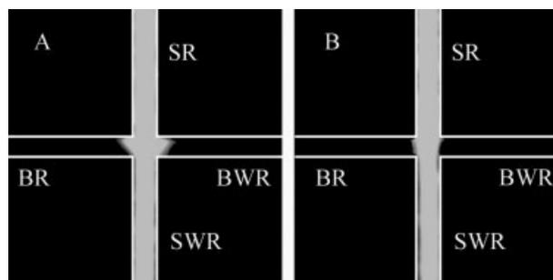
**Figure 3.** Fluorescence images of sample loading profile with different liquid height in SR with tilted angle of  $17^\circ$  after 100 s injection. (A) Sample liquid level 0.30 cm height and (B) sample liquid level 0.27 cm height.
