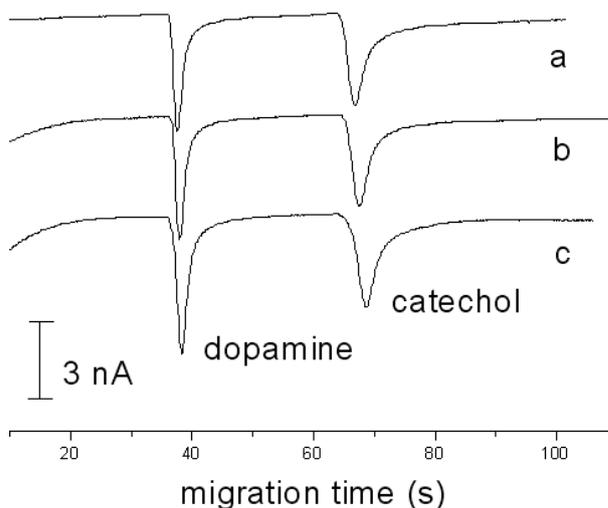
**Figure 4.** Electropherograms for the separation of 500  $\mu\text{M}$  of dopamine and catechol with different tilted angle injection, sample loading time: 100 s. (a)  $30^\circ$  ( $\Delta H = 0.50$  cm); (b)  $17^\circ$  ( $\Delta H = 0.30$  cm) and (c)  $9^\circ$  ( $\Delta H = 0.15$  cm).
