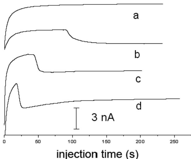
**Figure 5.** Measured current of 500  $\mu\text{M}$  dopamine at the SWR exit as a function of injection time. The microfluidic flow was generated by differential hydrostatic pressure between SR and SWR with different tilted angles. (a) 17° tilted angle, with blank solution injection; (b) 9° tilted angle; (c) 17° tilted angle; (d) 30° tilted angle. Detection potential: +1.4 V.
