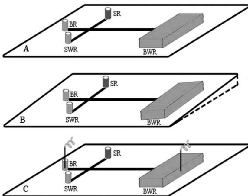
**Figure 1.** Scheme of microchip status in the process of injection. (A) Before injection, four reservoirs were filled with desired solution; (B) in injection stage, the microchip was tilted and the sample was driven to pass through the injection channel; (C) after sample loading, the microchip was levelled and separation voltage was applied.
