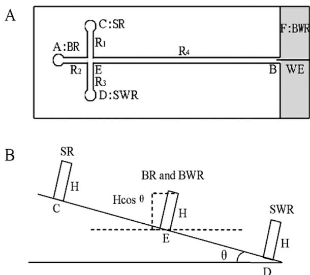
**Figure 2.** (A) Schematic drawing of the simple crosschannel microchip used in the present work and (B) side view of the tilted microchip.
