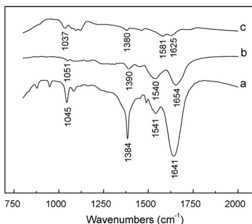
Fig. 3. FT-IR spectra of Mb-TiO<sub>2</sub>/MWCNTs (a), free Mb (b), TiO<sub>2</sub>/MWCNTs and film (c).
