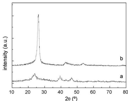
Fig. 2. XRD pattern of TiO<sub>2</sub>/MWCNTs (a) and acid-treated MWCNTs (b).
