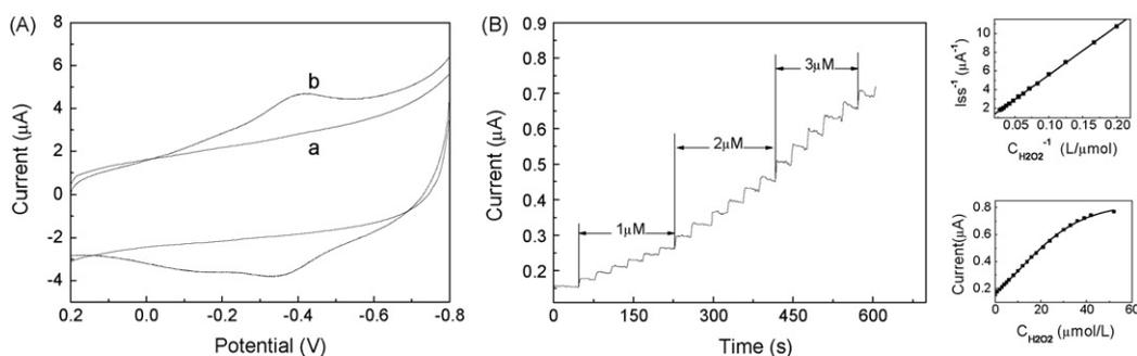
Fig. 4. (A) CVs of the bare GC electrode (a) and Mb-TiO<sub>2</sub>/MWCNTs modified GC electrode (b) in pH 7.0 PBS. Scan rate 100 mV/s. (B) Amperometric response of Mb-TiO<sub>2</sub>/MWCNTs modified GC electrode with successive addition of H<sub>2</sub>O<sub>2</sub> to the 0.1 mol/L pH 7.0 PBS under string. The applied potential is -0.4 V.
