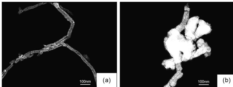
Fig. 1. TEM images of A-MWCNTs (a) and  $\text{TiO}_2$ /MWCNTs composites (b).
