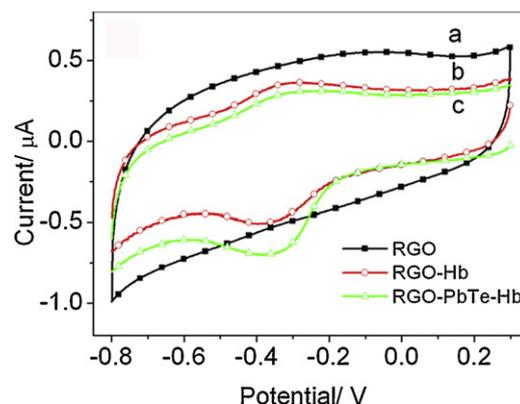
Fig. 3. Cyclic voltammograms of (a) RGO/GCE, (b) RGO-Hb/GCE, and (c) RGO-PbTe-Hb/GCE at a scan rate of  $100 \text{ mV s}^{-1}$ .
