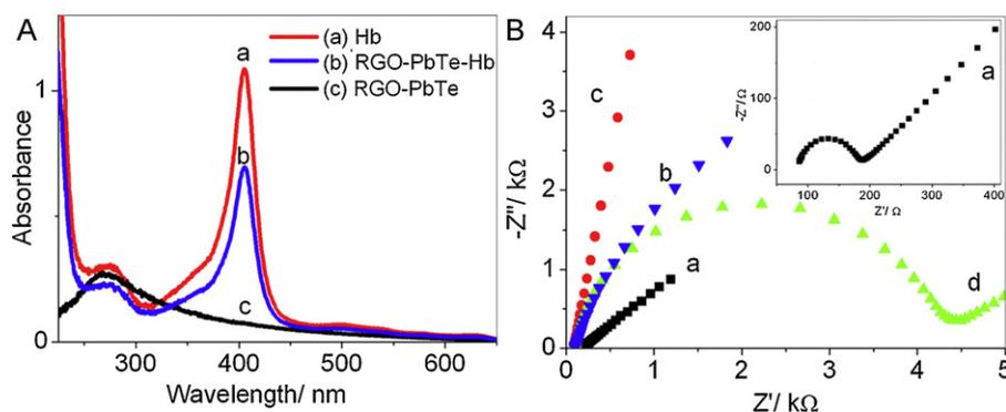
Fig. 2. (A) UV-vis spectra of (a) Hb, (b) RGO-PbTe-Hb, and (c) RGO-PbTe in 0.1 M pH 7.0 PBS. (B) Nyquist plots of modified GCE recorded in solution containing 0.1 M KCl and 10 mM  $\text{Fe}(\text{CN})_6^{3-}/\text{Fe}(\text{CN})_6^{4-}$ : (a) bare GCE, (b) RGO/GCE, (c) RGO-PbTe/GCE, and (d) RGO-PbTe-Hb/GCE.
