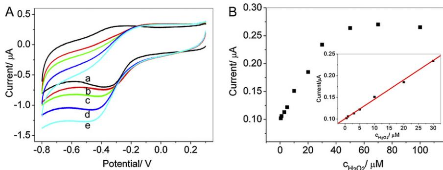
**Fig. 4.** (A) Cyclic voltammograms of the RGO–PbTe–Hb at a scan rate of  $100 \text{ mV s}^{-1}$  in  $0.1 \text{ M}$  pH  $7.0$  PBS solutions with (a)  $0$ , (b)  $5.0$ , (c)  $10.0$ , (d)  $30.0$ , (e)  $50.0 \mu\text{M}$   $\text{H}_2\text{O}_2$ . (B) Plots of the electrocatalytic current ( $i$ ) vs.  $\text{H}_2\text{O}_2$  concentration. Inset: linear plots of  $i$  vs.  $\text{H}_2\text{O}_2$  concentration.
