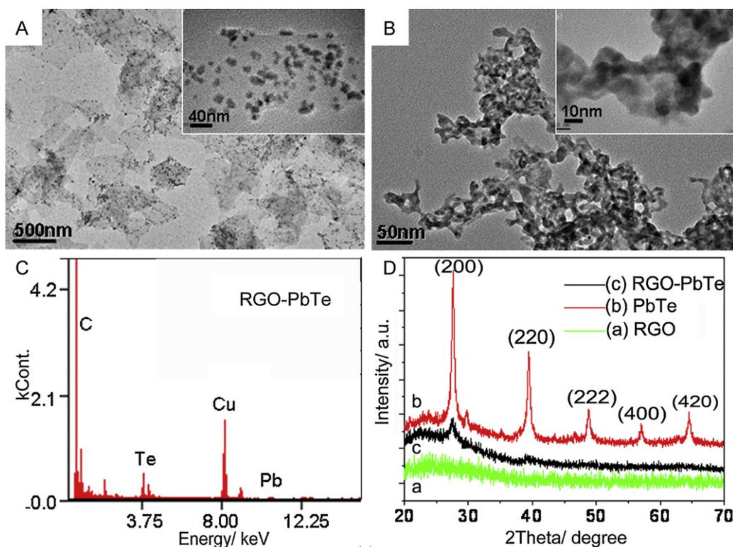
Fig. 1. TEM images of RGO-PbTe (A) and PbTe (B), EDS of the RGO-PbTe (C), and the XRD patterns (D) of the (a) RGO, (b) PbTe, and (c) RGO-PbTe.
