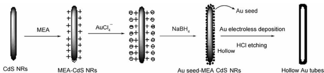
**Scheme 1** Schematic representation of the formation of CdS-nanorod/Au-nanoparticle composite and Au hollow tubes.
