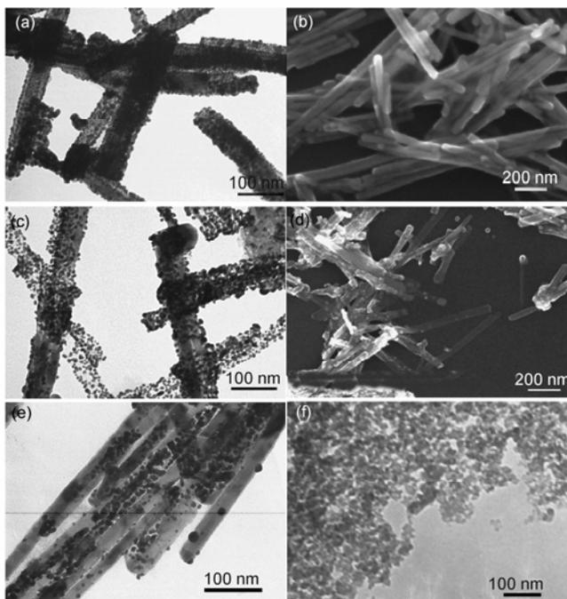
**Figure 2** TEM and SEM images of CdS-MEA/Au nanorods after Au electroless deposition ((a), (b)) and Au hollow tubes produced by HCl treatment ((c), (d)). (e) is the TEM image of unmodified CdS nanorods with Au nanoparticles after electroless deposition and (f) is the TEM image of the random Au nanoparticles produced by HCl treatment of CdS-MEA/Au nanorods without Au electroless deposition.
