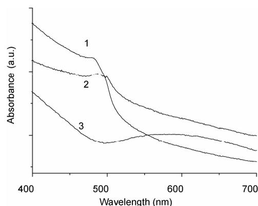
**Figure 4** UV-Vis spectra of the aqueous dispersion of pure CdS nanorods (line 1), CdS-MEA/Au nanorods (line 2) and hollow Au tubes after dissolving the inner CdS core by HCl (line 3).
