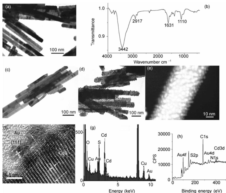
**Figure 1** (a) TEM image of MEA modified CdS nanorods; (b) IR spectrum of MEA modified CdS nanorods; (c) TEM image of unmodified CdS nanorods after Au deposition; (d) TEM image of MEA modified CdS nanorods after Au deposition; (e) an enlarged dark field image of CdS-MEA nanorods/Au-nanoparticles; (f) the corresponding HRTEM image of (e); (g) the corresponding EDS of (e); and (h) XPS spectrum for CdS-MEA nanorods/Au-nanoparticles.
