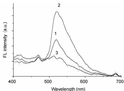
**Figure 3** FL spectra of aqueous dispersion of pure CdS nanorods (line 1), MEA modified CdS nanorods (line 2), and CdS-MEA/Au nanorods (line 3) (excitation at 360 nm).
