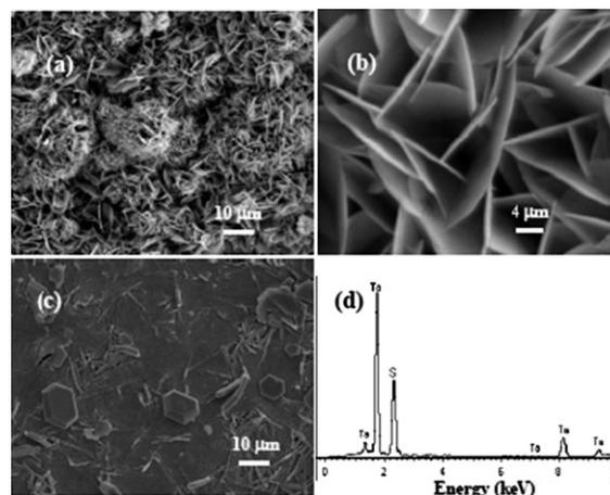
**Fig. 4** (a, b) SEM image of nanosheets prepared with 120 mg of iodine. (c) SEM image of the products prepared without iodine. (d) EDX spectrum of the microplate in Fig. 4(c).
