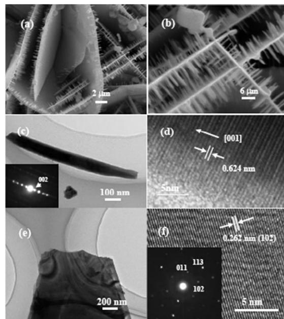
**Fig. 3** Microstructures of the products prepared with 60 mg of iodine. (a, b) SEM images. (c) TEM image and SAED pattern (inset) of a single nanorod. (d) HRTEM image of the nanorod in (c). (e) TEM image of a nanosheet. (f) HRTEM image and SAED pattern (inset) of the nanosheet in (e).
