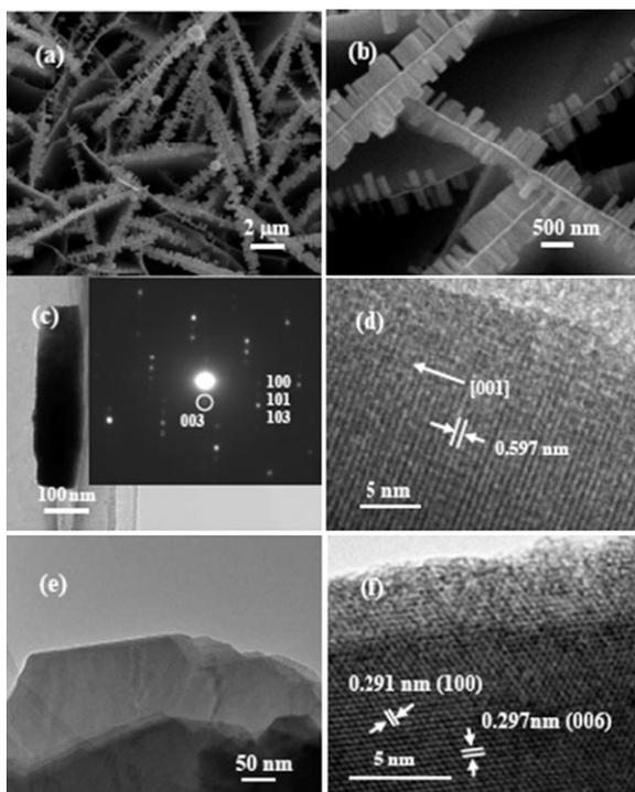
**Fig. 2** Microstructures of the products prepared with 30 mg of iodine. (a, b) SEM image (overview). (c) TEM image and SAED pattern (inset) of a single nanorod. (d) HRTEM image of the nanorod in (c). (e) TEM image of a nanosheet. (f) HRTEM image of the nanosheet in (e).
