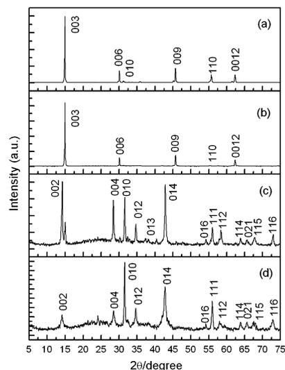
**Fig. 1** Powder XRD patterns of the products prepared by chemical vapor transport with iodine: (a) 0.0, (b) 30, (c) 60, and (d) 120 mg at  $750^\circ\text{C}$  for 6 h. The peaks which are not indexed in (c) can be attributed to the reflections of 3R- $\text{TaS}_2$ . The peak which is not indexed in (d) is an unknown impurity peak with the main phase of sample 4 being the 2H- $\text{TaS}_2$  structure.
