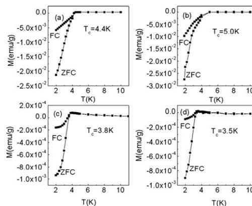
**Fig. 6** DC magnetization as a function of temperature for the products prepared with (a) 0.0, (b) 30, (c) 60 and (d) 120 mg of iodine, under conditions of zero-field cooling (ZFC) and field cooling (FC) at 50 Oe.
