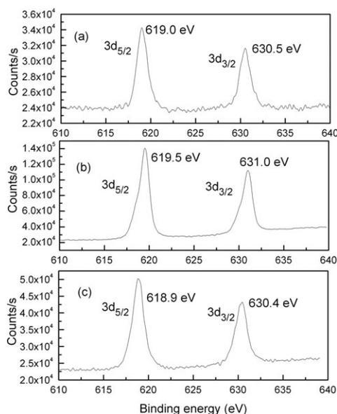
**Fig. 5** I 3d binding energy spectra of the samples prepared with (a) 30, (b) 60 and (c) 120 mg of iodine, respectively.
