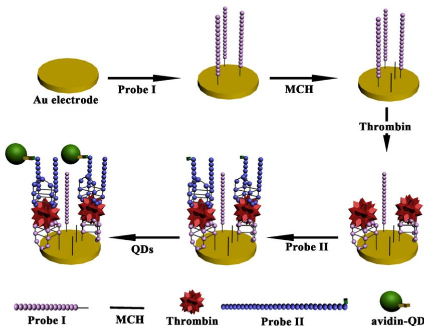
Fig. 1. Schematic diagram for the biosensor fabrication.
