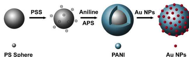
**Scheme 1.** Schematic illustration of the synthesis of complex PS/PANI/Au.
