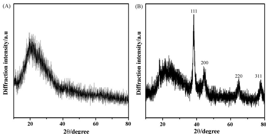
Fig. 2. The XRD patterns of the PS/PANI nanocomposite (A) and the PS/PANI/Au nanocomposite (B).
