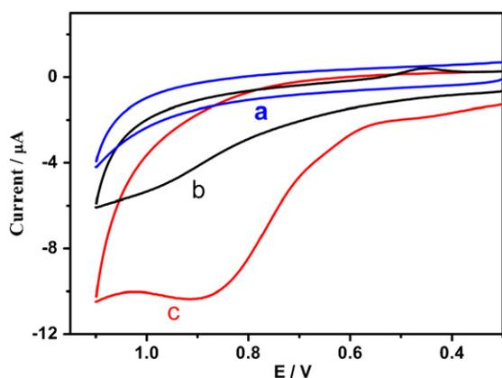
Fig. 3. Cyclic voltammograms of bare GCE (a), PS/PANI/Au/GCE (b), and cells/PS/PANI/Au/GCE (c) in pH 7.4 PBS. Scan rate: 50 mV s<sup>-1</sup>.
