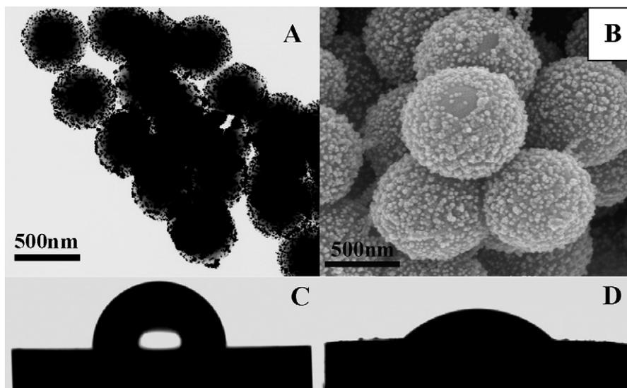
**Fig. 1.** (A) TEM and (B) SEM images of the PS/PANI/Au nanocomposite. Contact angle of bare electrode (C) and PS/PANI/Au modified electrode (D).
