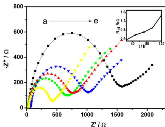
**Fig. 5.** EIS measurements of HL-60 cells proliferated on PS/PANI/Au/GCE after cell incubation for (a) 24 h, (b) 48 h, (c) 72 h, (d) 96 h and (e) 120 h. Inset: relationship between electron transfer resistance and proliferation time of HL-60 cells on PS/PANI/Au/GCE.
