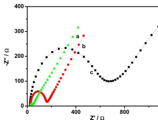
Fig. 4. Nyquist diagrams of electrochemical impedance spectra of bare GCE (a), PS/PANI/Au/GCE (b), and cells/PS/PANI/Au/GCE (c).
