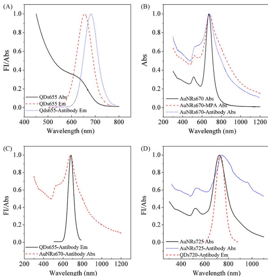
**Fig. 2.** Normalized fluorescence spectra of Mn: CdTe Qdots and absorption spectra of AuNRs. (A) Mn: CdTe655 before and after labeled with goat anti-human IgG. (B) AuNRs670 before and after SAM formation, AuNRs670 after labeled with rabbit anti-human IgG. (C) Overlap spectra of the Mn: CdTe655-Ab1 and AuNRs670-Ab2. (D) Mn: CdTe720 labeled with goat anti-human IgG, AuNRs725 before and after labeled with rabbit anti-human IgG.
