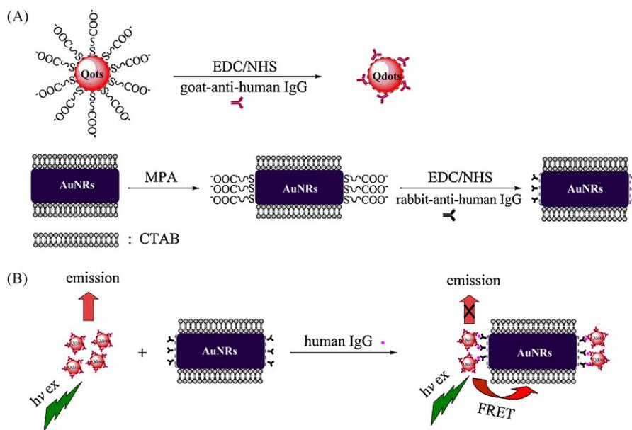
**Fig. 1.** (A) Schematic illustration of antibody immobilized on the surface of Mn:CdTe Qdots and AuNRs with EDC/NHS. (B) Schematic illustration of the FRET system between Qdots and AuNRs. See text for details.
