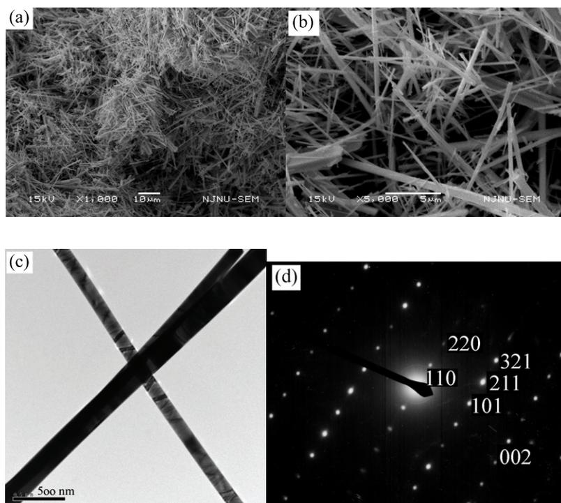
**Figure 6.** SEM ((a), (b)) and TEM (c) images and SAED pattern (d) of as-prepared  $\text{Sb}_2\text{Se}_3$ .
