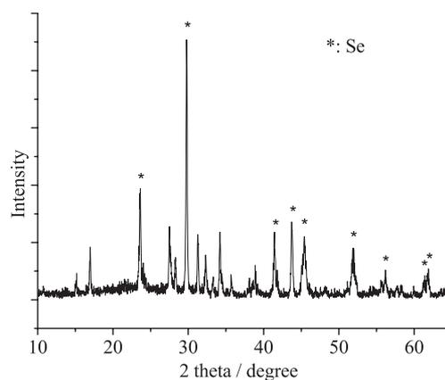
Figure 2. XRD pattern of the sample obtained after 1 h of reaction.
