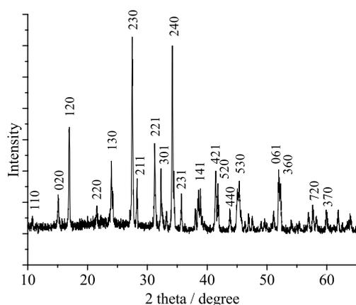
Figure 1. XRD pattern of as-prepared  $\text{Sb}_2\text{Se}_3$ .
