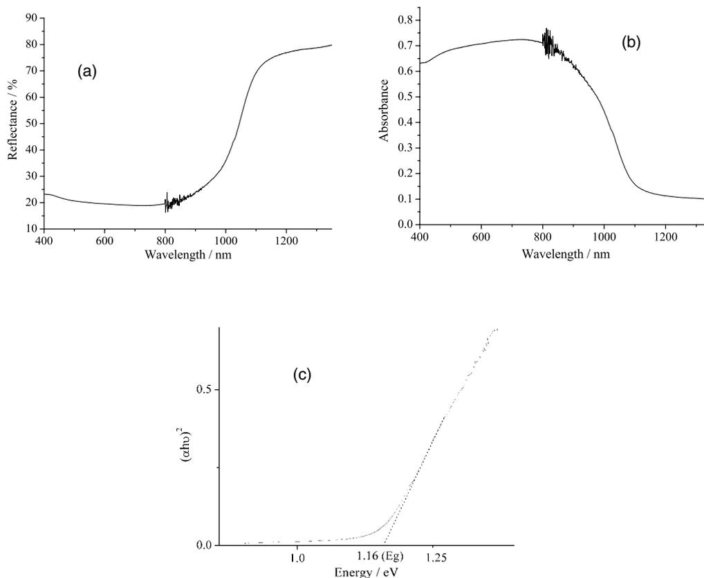
**Figure 7.** (a) The diffuse reflectance spectrum of as-prepared  $\text{Sb}_2\text{Se}_3$  submicron rods; (b) the absorbance spectrum corresponding to (a); (c) the plot corresponding to (b), from which the bandgap ( $E_g$ ) can be derived to be 1.16 eV.
