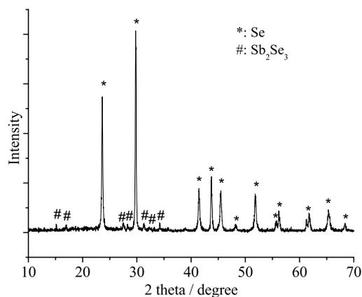
**Figure 5.** XRD pattern of the sample obtained solvothermally at 180 °C after 30 h of reaction.
