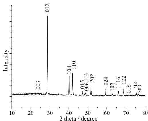
**Figure 3.** XRD pattern of the sample obtained when NaOH was added.
