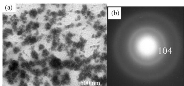
**Figure 4.** TEM image (a) and SAED pattern (b) of the Sb colloid.
