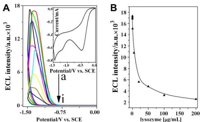
**Fig. 3.** (A) The ECL-potential curves of the lysozyme biosensor with different protein concentrations ( $\mu\text{g/mL}$ ): (a) 0, (b) 0.1, (c) 0.2, (d) 0.5, (e) 2, (f) 5, (g) 20, (h) 100, (i) 200. The insert shows the cyclic voltammetry response of curve a during the ECL measurement. (B) The ECL-concentration curve draws from (A).
