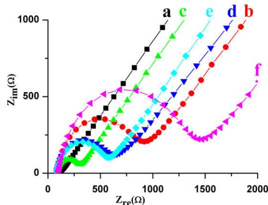
Fig. 2. EIS of the electrode at different stages in 0.1 mol/L KCl and 2 mmol/L  $\text{Fe}(\text{CN})_6^{3-}/\text{Fe}(\text{CN})_6^{4-}$ . (a) Bare Au electrode, (b) probe/Au electrode, (c) lysozyme/probe/Au electrode, (d) cDNA/lysozyme/probe/Au electrode, (e) QDs/cDNA/lysozyme/probe/Au electrode, and (f) cDNA/probe/Au electrode.
