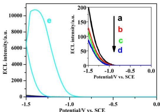
**Fig. 4.** Electrochemiluminescence intensity versus potential. (a) Bare Au electrode, (b) probe/Au electrode, (c) lysozyme/probe/Au electrode, (d) cDNA/lysozyme/probe/Au electrode, (e) QDs/cDNA/lysozyme/probe/Au electrode. The inset is the amplification form of curve (a), (b), (c) and (d).
