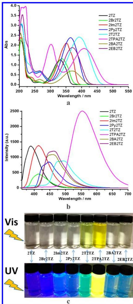
**Figure 1.** UV-vis absorption spectra (a), fluorescence emission excited at 350 nm (b), and their visual photographs (c) for the heterocyclic aromatic compounds in their methanol solutions at room temperature with the same concentration of  $5.0 \times 10^{-5} \text{ mol}\cdot\text{L}^{-1}$ .
