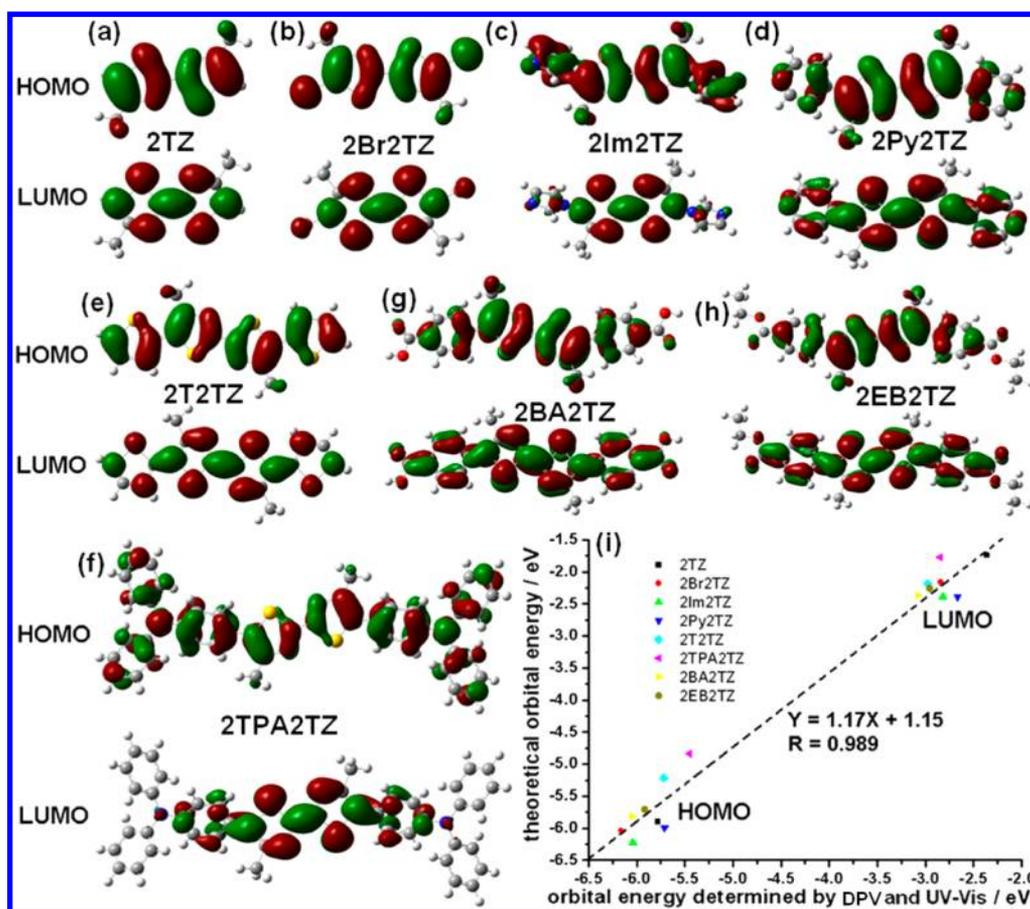
**Figure 6.** HOMOs and LUMOs of 2TZ (a), 2Br2TZ (b), 2Im2TZ (c), 2Py2TZ (d), 2T2TZ (e), 2TPA2TZ (f), 2BA2TZ (g), and 2EB2TZ (h) calculated with B3LYP/6-31G\*. (i) Energy level correlation between the DPV, UV-vis absorption spectra, and the computational data.
