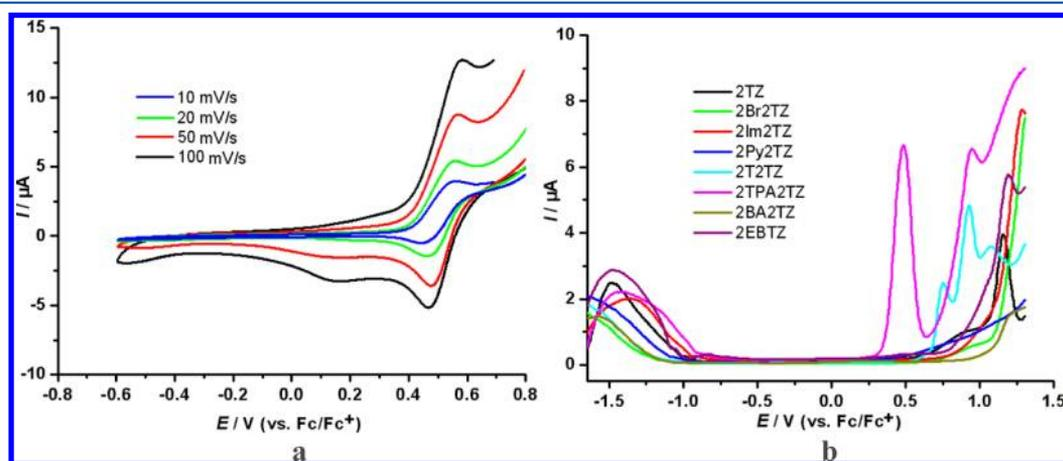
**Figure 5.** CV (a) and DPV (b) for related heterocyclic aromatic compounds in  $\text{CH}_2\text{Cl}_2$  ( $1.0 \times 10^{-3} \text{ mol}\cdot\text{L}^{-1}$ ) containing  $0.10 \text{ mol}\cdot\text{L}^{-1}$  of  $\text{TBAClO}_4$  under argon. In (a), different scanning rates of 10, 20, 50, and 100 mV/s are used for 2TPA2TZ vs  $\text{Fc}/\text{Fc}^+$ .
