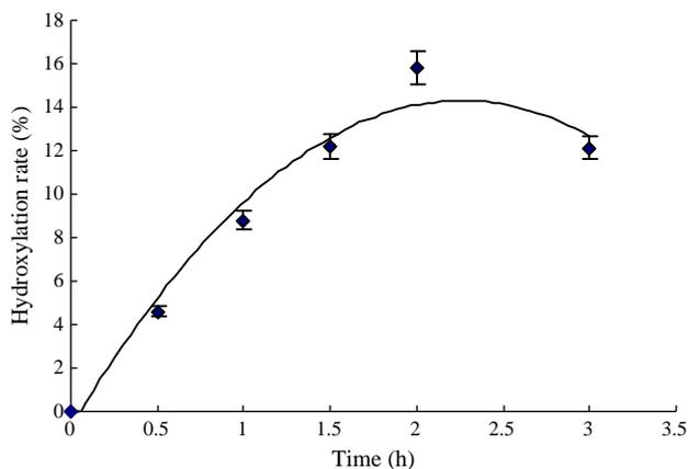
**Fig. 6.** Effect of incubation time on hydroxylation rate. The reaction mixture (100  $\mu$ L), containing 14  $\mu$ g PHD3, 1.0 mM DTT, 2.0 mM ascorbate, 50  $\mu$ M FeSO<sub>4</sub>, 0.16 mM 2-oxoglutarate, 2.0 mg/mL BSA, 0.60 mg/mL catalase, and 66.55  $\mu$ M HIF-1 $\alpha$  peptide in 20 mM phosphate buffer (pH 7.0) was incubated at 37  $^{\circ}$ C for 0, 30, 60, 90, 120, and 180 min. The data shown are means and standard deviations of three independent experiments.
