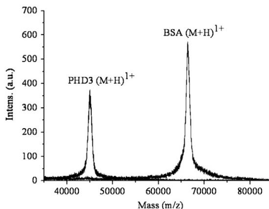
Fig. 3. Matrix-assisted laser desorption/ionization time of flight mass spectral analysis of purified recombinant human PHD3. The results are the average of three determinations. Bovine serum albumin (BSA) was used as a standard protein.
