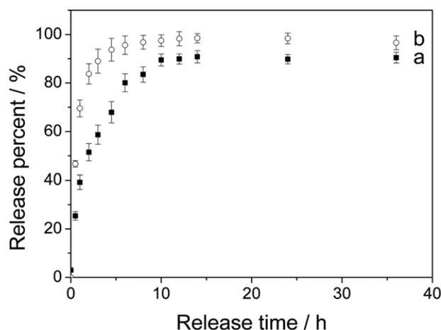
**Figure 7.** Release profiles of ASP from ASP-loaded magnetic MIPs (a) and magnetic NIPs (b) in pH 6.8 PBS solution.
