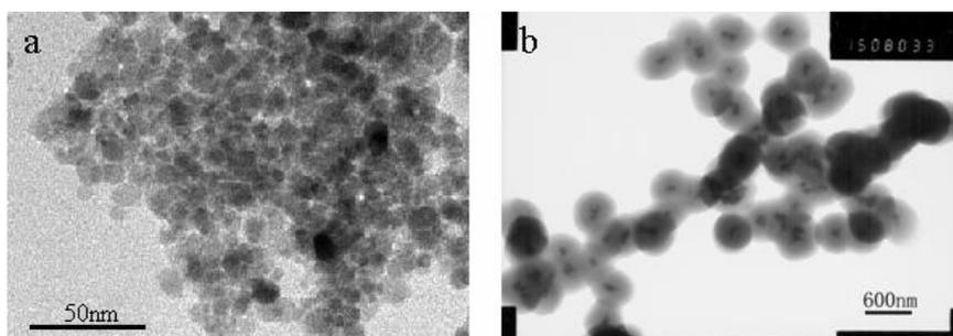
**Figure 3.** TEM images of  $\text{Fe}_3\text{O}_4$  nanoparticles (a) and magnetic MIPs (b).
