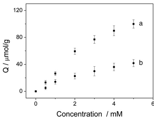
**Figure 6.** Adsorption isotherms of ASP on magnetic MIPs (a) and on magnetic NIPs (b). Amount of polymers: 20 mg, volume: 2.0 ml.
