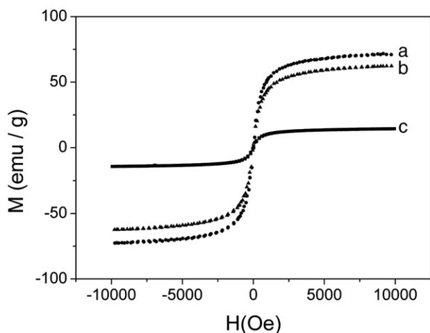
**Figure 5.** Magnetization curves obtained by VSM at room temperature of Fe<sub>3</sub>O<sub>4</sub> (a), double-bond-functionalized Fe<sub>3</sub>O<sub>4</sub> (b) and magnetic MIPs (c).
