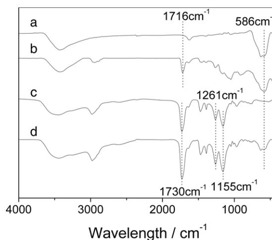
**Figure 1.** FTIR spectra of the  $Fe_3O_4$  (a), double-bond-functionalized  $Fe_3O_4$  (b), pure MIPs (c) and magnetic MIPs (d).
