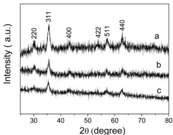
**Figure 2.** X-ray diffraction patterns of  $\text{Fe}_3\text{O}_4$  (a), double-bond-functionalized  $\text{Fe}_3\text{O}_4$  (b) and magnetic MIPs (c).
