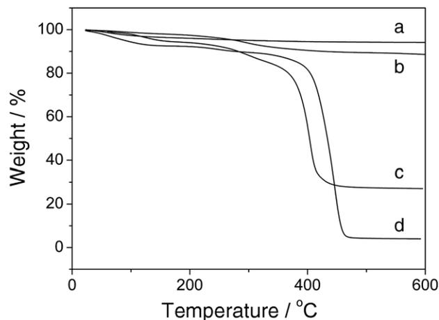
**Figure 4.** TGA curves of  $\text{Fe}_3\text{O}_4$  (a), double-bond-functionalized  $\text{Fe}_3\text{O}_4$  (b), magnetic MIPs (c) and pure MIPs (d).
