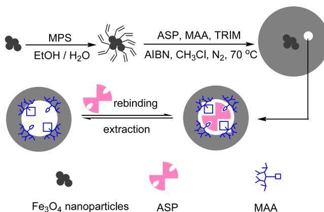
**Scheme 1.** Schematic illustration of the synthesis of magnetic MIPs.
