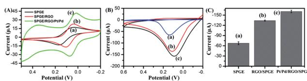
Fig. 3 (A) Cyclic voltammograms of SPGE (a), RGO/SPGE (b), Pt/Pd/RGO/SPGE (c) in 1 mM  $K_3Fe(CN)_6$  at a scan rate of  $100 \text{ mV s}^{-1}$ . (B) Cyclic voltammograms of *p*-NP in 5 mM *p*-NPP solution containing  $10 \mu\text{L}$ ,  $0.1 \text{ mg mL}^{-1}$  ALP using SPGE (a), RGO/SPGE (b) and Pt/Pd/RGO/SPGE (c) electrode respectively. (C) The peak values of the current in (B). (a) 0.138 V, (b) 0.113 V, and (c) 0.086 V.
