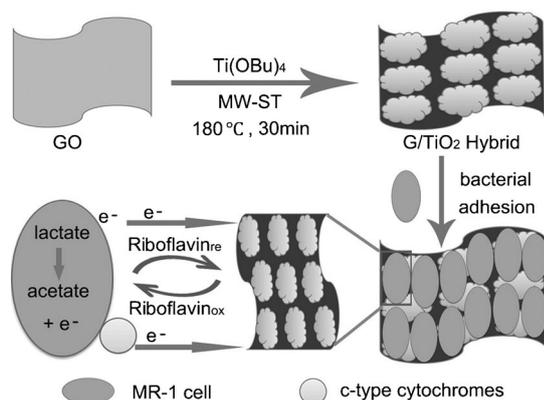
**Scheme 1.** Synthesis of nanostructured G/TiO<sub>2</sub> hybrids by a one-pot MWST process and their use as MFC anode materials.
