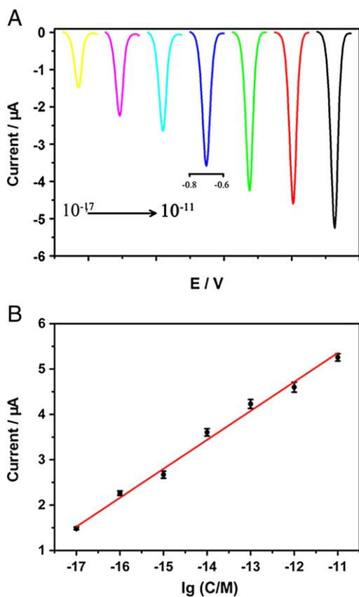
**Fig. 3.** (A) ASV signal of  $\text{Cd}^{2+}$  responding to  $10^{-17}$ ,  $10^{-16}$ ,  $10^{-15}$ ,  $10^{-14}$ ,  $10^{-13}$ ,  $10^{-12}$ , and  $10^{-11}$  M miR-16 (left to right). (B) The quantitative linear dynamic range of the designed method.
