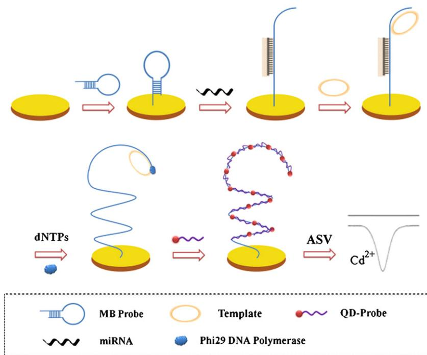
Fig. 1. Schematic representation of the designed strategy for miRNA detection.
