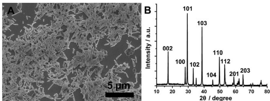
**Fig. 1** SEM image (a) and XRD patterns(b) of Cd(OH)Cl nanorods
