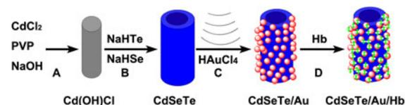
**Scheme 1** Schematic illustration of the fabrication process of the CdSe<sub>x</sub>Te<sub>1-x</sub>/Au/Hb biocomposites. *a* Synthesis of Cd(OH)Cl nanorods. *b* Preparation of CdSe<sub>x</sub>Te<sub>1-x</sub> nanotubes. *c* In situ decoration of AuNPs via a sonochemical method. *d* Assembly of Hb on the CdSe<sub>x</sub>Te<sub>1-x</sub>/Au nanocomposite
