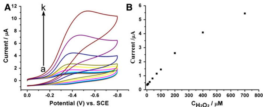
**Fig. 6** Cyclic voltammograms (a) and the calibration curve (b) of CdSe<sub>x</sub>Te<sub>1-x</sub>/Au/Hb modified GCEs in 0.1 M PBS at pH = 7.0 in the presence of: (a) 2, (b) 4, (c) 7, (d) 10, (e) 20, (f) 40, (g) 70, (h) 100, (i) 200, (j) 400, and (k) 700 mM H<sub>2</sub>O<sub>2</sub> at a scan rate of 200 mV s<sup>-1</sup>
