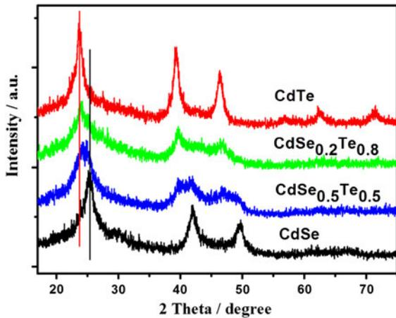
**Fig. 3** XRD patterns of CdTe, CdSe, and CdSe<sub>x</sub>Te<sub>1-x</sub> nanotubes with different ratios of selenium and tellurium. The percentages indicate the initial concentrations of Se and Te. The vertical lines represent XRD patterns of bulk CdTe (bottom, JCPDS 75-2086) and CdSe (top, JCPDS 19-0191)
