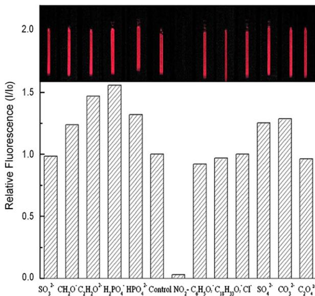
**Fig. 2.** Relative fluorescence ( $I/I_0$ ) of BSA-AuNCs solution in the presence of 50  $\mu\text{M}$  various anions. Inset: Photographs of BSA-AuNCs solution in the presence of 50  $\mu\text{M}$  various anion under UV light.
