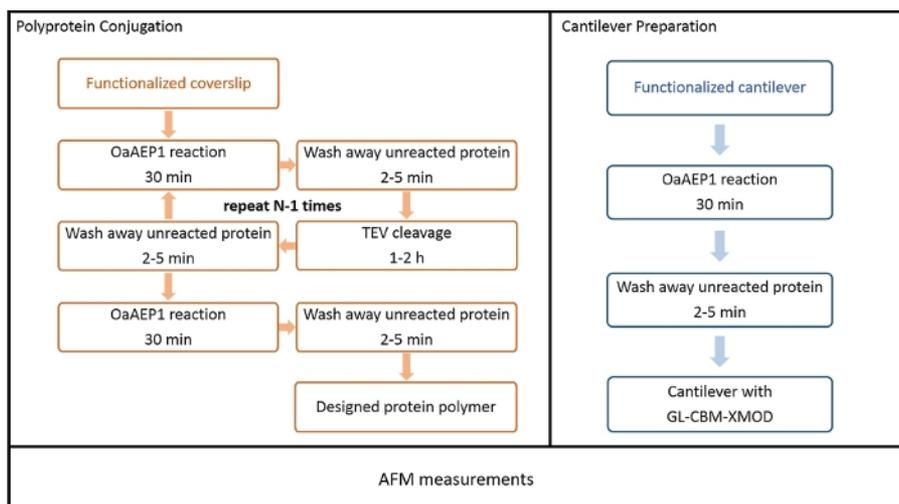
**Figure 5: Process chart describing each step for polyprotein immobilization on the surface.** Top left process flow diagram shows the stepwise building of polyprotein with controlled sequences on the coverslip. Top right diagram shows the preparation of the functionalized cantilever used in the AFM measurements. [Please click here to view a larger version of this figure.](#)
