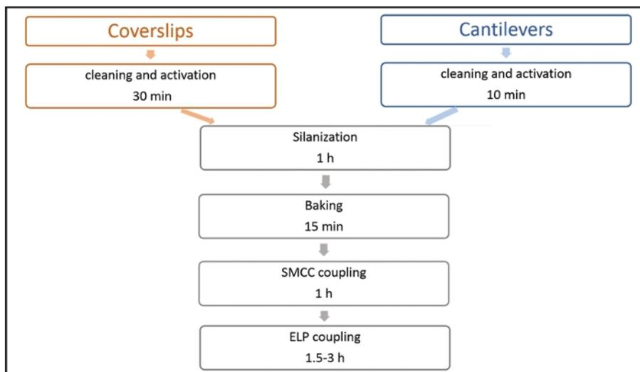
**Figure 4: Process chart describing each step for functionalizing glass coverslips and cantilever.** After cleaning and activation by chromic acid, coverslip and cantilever share similar functionalization process, except the last step in which GL-ELP<sub>50nm</sub>-C couples with coverslip while C-ELP<sub>50nm</sub>-NGL couples with cantilever. [Please click here to view a larger version of this figure.](#)
