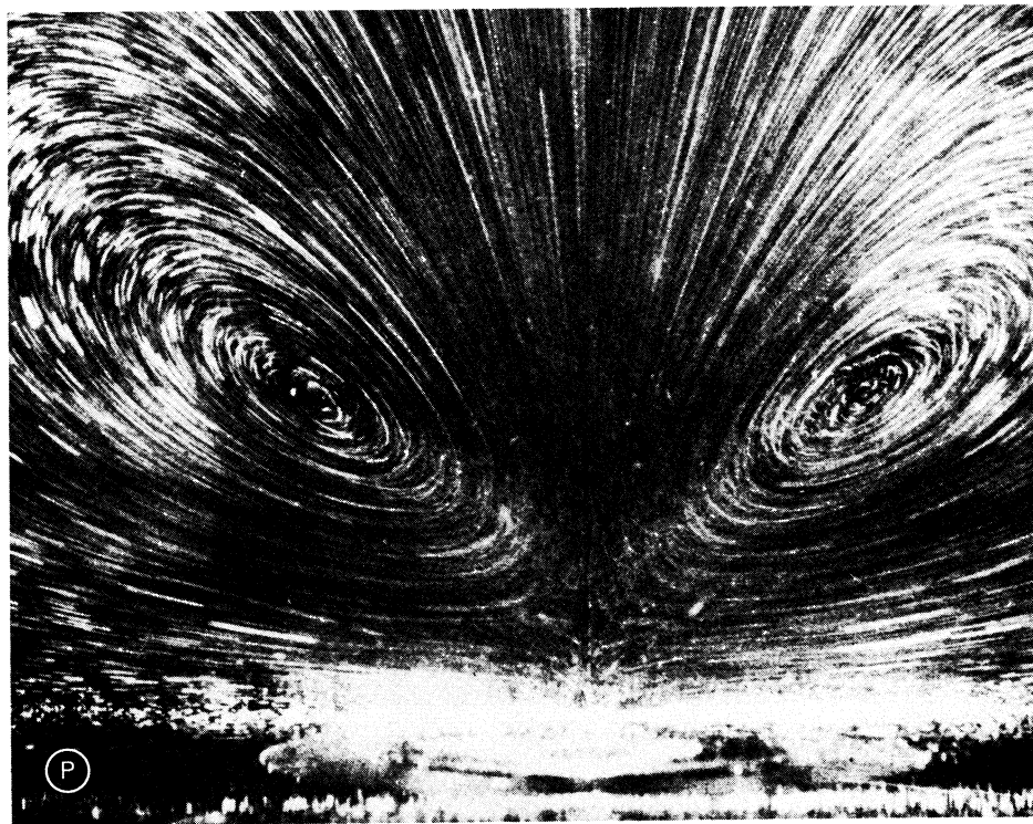
FIGURE 2.5-6. Velocity fields near a sudden contraction. The fluid moves from top to bottom in the photographs from a large reservoir into a small circular tube. (N) The streamlines in glycerin are straight and all directed toward the exit; (P) a 1.67% aqueous polyacrylamide solution shows a large toroidal vortex. [Photographs by H. Giesekus, given in A. B. Metzner, E. A. Uebler, and C. F. Chan Man Fong, AIChE J. , 15, 750-758 (1969).]
