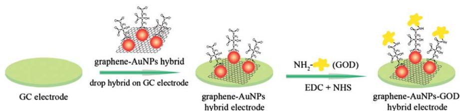
**Scheme 2** Schematic diagram of fabricating the model of the amperometric glucose biosensor.
