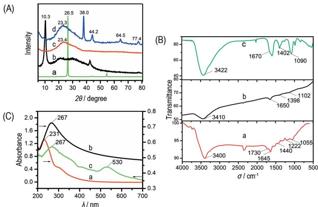
**Fig. 1** (A) XRD patterns of (a) graphite, (b) GO, (c) graphene, and (d) graphene–AuNPs hybrid. (B) FT-IR spectra of (a) GO, (b) graphene, and (c) graphene–AuNPs hybrid. (C) UV-Vis absorption spectra of (a) GO, (b) graphene, and (c) graphene–AuNPs hybrid.
