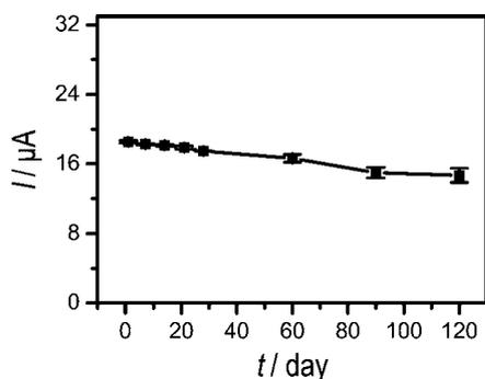
**Fig. 10** The relationship of the reduction peak currents of the GOD bound and the time for storage. Error bars =  $\pm$  standard deviation. Every point was an average value of the three model of the biosensors for independent measurements.
