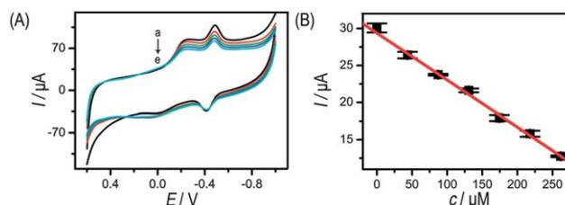
**Fig. 9** (A) CVs of the model of the biosensor in standard human serum sample solutions containing (a) 0 μM, (b) 87.2 μM, (c) 130.8 μM, (d) 174.4 μM, and (e) 218 μM glucose. (B) The calibration curve of the response currents *versus* the glucose concentrations in standard human serum sample. *R* = 0.998. Error bars = ± standard deviation. Every point was an average value of three model of the biosensors for independent measurements.
