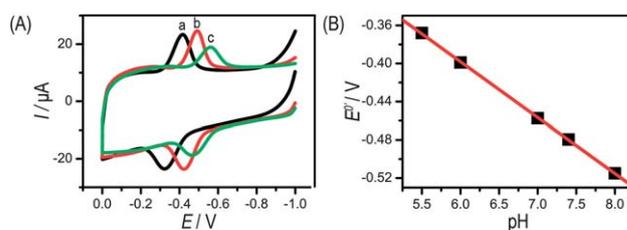
**Fig. 6** (A) CVs of the graphene–AuNPs–GOD hybrid electrode in 0.1 M PBS with different pH values of (a) 5.5, (b) 7.0, and (c) 8.0 at the scan rate of 50  $\text{mV s}^{-1}$ . (B) The relationship of  $E^{\text{v}}$  versus pH.
