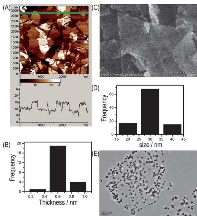
**Fig. 2** (A) AFM image of graphene, cross-section analysis was based on the chosen line. (B) The histogram displaying the distribution of sheet thicknesses measured on 20 different sheets from AFM results. (C) FESEM image of the graphene–AuNPs hybrid. (D) The histogram displaying the size distributions of the AuNPs on the surface of the graphene, calculated by 100 particles from FESEM results. (E) HRTEM image of the graphene–AuNPs hybrid.
