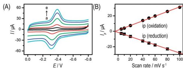
**Fig. 4** (A) CVs of the graphene–AuNPs–GOD hybrid electrode at different scan rates: (a) 10  $\text{mV s}^{-1}$ , (b) 20  $\text{mV s}^{-1}$ , (c) 50  $\text{mV s}^{-1}$ , (d) 80  $\text{mV s}^{-1}$ , and (e) 100  $\text{mV s}^{-1}$ . (B) Plot of redox peak currents versus various scan rates from 5  $\text{mV s}^{-1}$  to 100  $\text{mV s}^{-1}$ .
