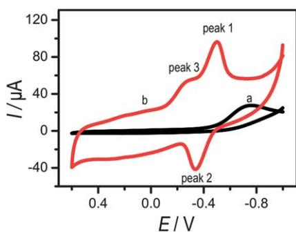
**Fig. 7** CVs of (a) GC electrode and (b) graphene-AuNPs-GOD hybrid electrode in 0.1 M PBS solution (pH 5.5) saturated with O<sub>2</sub> at the scan rate of 50 mV s<sup>-1</sup>.
