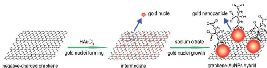
Scheme 1 Schematic diagram of synthesizing the graphene–AuNPs hybrid.
