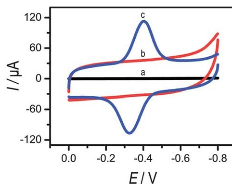
**Fig. 3** CVs of (a) GC electrode, (b) graphene–AuNPs hybrid electrode, and (c) graphene–AuNPs–GOD hybrid electrode in 0.1 M PBS solution (pH 5.5) saturated with  $\text{N}_2$  at the scan rate of  $50 \text{ mV s}^{-1}$ .
