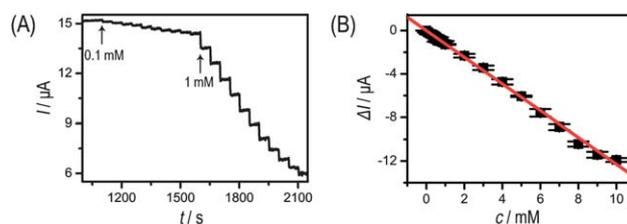
**Fig. 8** (A) *I-t* curve of the model of the biosensor for successive additions of specific concentrations of glucose to 0.1 M PBS solution (pH 5.5) which was saturated with O<sub>2</sub>. The testing solution was kept stirring. Applied potential: -0.2 V. (B) The relationship of the response current *versus* the glucose concentration. *R* = 0.999. Error bars = ± standard deviation. Every point was an average value of three model of the biosensors for independent measurements.
