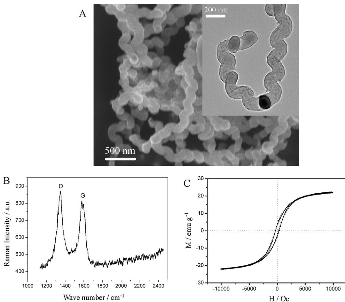
**Fig. 1.** (A) Typical FESEM image of the PDDA-HCNTs, (B) Raman spectra and (C) magnetization curve of the PDDA-HCNTs. Inset: TEM image of the PDDA-HCNTs.
