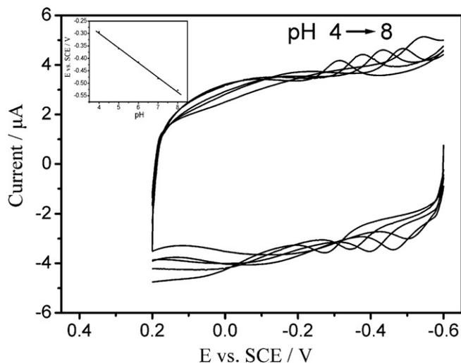
**Fig. 4.** The CVs of the GOD-PDDA-HCNTs/MGCE in different pH solutions.
