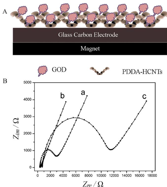
Fig. 2. (A) Schematic of glucose detection by electrochemical method using PDDA-HCNTs modified MGCE. (B) EIS of bare (a), PDDA-HCNTs (b), and GOD-PDDA-HCNTs (c) modified MGCE in 0.10 M KCl containing 5.0 mM  $\text{K}_3[\text{Fe}(\text{CN})_6]/\text{K}_4[\text{Fe}(\text{CN})_6]$ .
