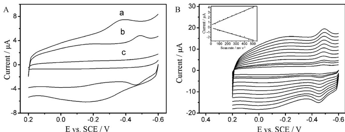
**Fig. 3.** (A) The CVs of different electrodes in nitrogen-saturated 0.1 M PBS (pH 7.0) at the scan rate of 100 mV/s: PDDA-HCNTs/MGCE (a), GOD-PDDA-HCNTs/MGCE (b) and GOD/MGCE (c). (B) The CVs of GOD-PDDA-HCNTs modified MGCE at scan rate of 50, 80, 100, 150, 200, 250, 300, 350, 400, 450, and 500 mV/s (from inner to outer curve) in nitrogen-saturated 0.10 M pH 7.0 PBS. Inset: plots of peak currents vs. scan rates.
