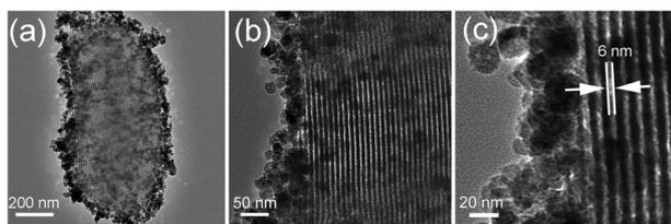
Fig. 1 TEM images of  $\text{Fe}_3\text{O}_4$ -SBA-15 hybrid.
