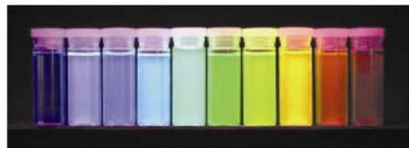
Figure 1 Ten distinguishable emission colors of ZnS-capped CdSe QDs excited with a near-UV lamp. From left to right (blue to red), the emission maxima are located at 443, 473, 481, 500, 518, 543, 565, 587, 610, and 655 nm [1].
