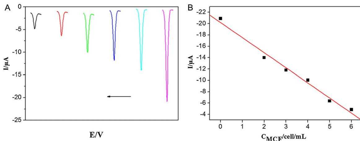
**Fig. 5.** Competition between cells and cDNA for binding to Apt-Qdots conjugates. A) Anodic stripping voltammograms of Qdots left at the modified gold electrode competing with 0,  $10^2$ ,  $10^3$ ,  $10^4$ ,  $10^5$  and  $10^6$  cells  $\text{mL}^{-1}$  (right to left). B) The corresponding linear calibration plot.
