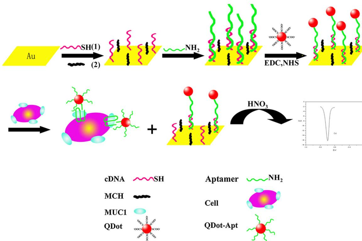
**Scheme 1.** Fabrication steps for the competitive electrochemical cytosensor.
