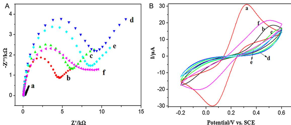
**Fig. 3.** (A) Nyquist diagrams of electrochemical impedance spectra recorded from 0.1 to  $10^5$  Hz for  $[\text{Fe}(\text{CN})_6]^{3-}/[\text{Fe}(\text{CN})_6]^{4-}$  (10 mM, 1:1) in 0.1 M KCl. (B) Cyclic Voltammograms at a bare Au electrode (a), cDNA/Au electrode (b), Apt/cDNA/Au electrode (c), Qdots/Apt/cDNA/Au electrode (d), MCF-7/Qdots/Apt/cDNA/Au electrode (e) and the final electrode after  $\text{HNO}_3$  dissolving (f).
