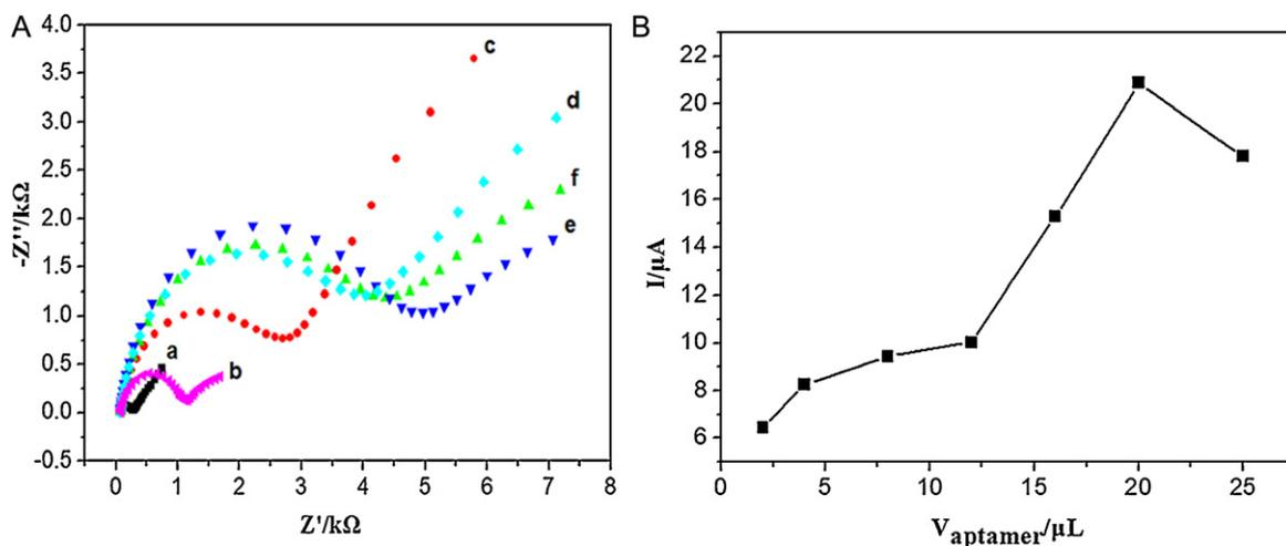
**Fig. 4.** (A) Nyquist diagrams of electrochemical impedance spectra recorded from 0.1 to  $10^5$  Hz for  $[\text{Fe}(\text{CN})_6]^{3-}/[\text{Fe}(\text{CN})_6]^{4-}$  (10 mM, 1:1) in 0.1 M KCl at a bare Au electrode (a), cDNA/Au electrode with the cDNA amount of 5, 10, 15, 20, 30  $\mu\text{L}$  (from curve b–f). (B) Effect of aptamer amount in electrode modification on peak current of Qdots/Apt/cDNA/Au electrode.
