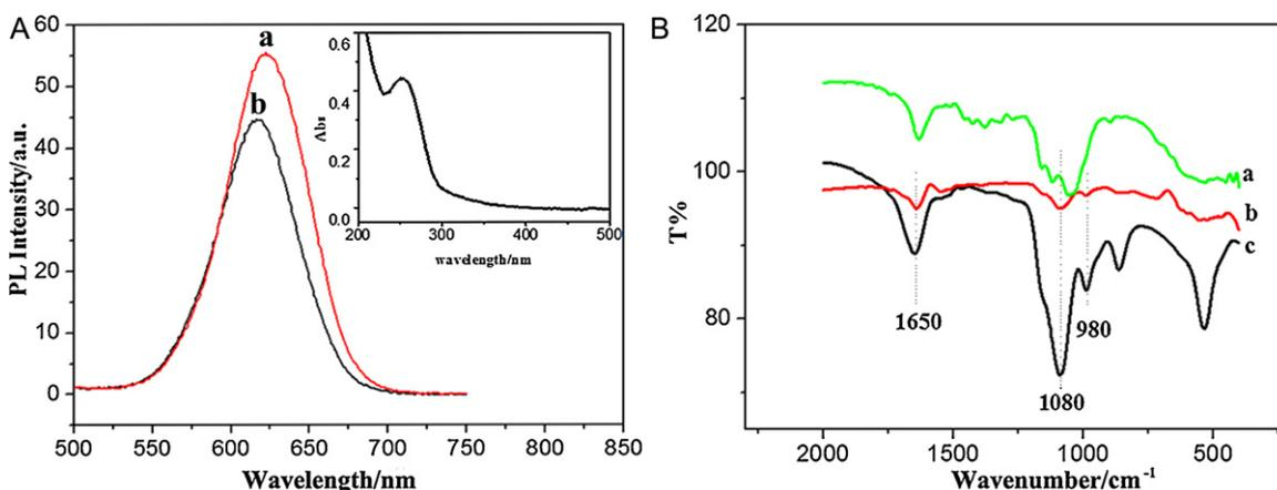
**Fig. 2.** (A) PL spectra of Qdots (a) and Apt-Qdots conjugates (b). Inset: UV-vis absorption spectrum of Apt-Qdots conjugates. (B) FTIR spectra of pure Qdots (a), Apt-Qdots conjugates (b) and pure aptamer (c).
