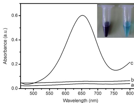
Figure 4. Typical absorption curves of TMB reaction solutions catalytically oxidized by the HCNTs in the presence of  $H_2O_2$  incubated at  $40^\circ\text{C}$  in pH 4.0 buffer: a)  $500$  mM  $H_2O_2$  without HCNTs, b)  $0$  mM  $H_2O_2$  with HCNTs, c)  $100$  mM  $H_2O_2$  with HCNTs. Inset: Images of the solutions of HCNTs (left) and the mixture of TMB and  $H_2O_2$  after catalytic reaction by HCNTs (right).
