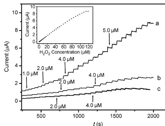
Figure 7. Amperometric responses of GCEs modified with HCNTs (a), l-HCNTs (b), and MWCNTs (c) at  $-0.40 \text{ V}$  upon successive additions of  $\text{H}_2\text{O}_2$  to  $0.1 \text{ M}$  pH 7.0 PBS at room temperature ( $25 \pm 2^\circ\text{C}$ ). Inset: plot of electrocatalytic current versus  $\text{H}_2\text{O}_2$  concentration at HCNTs-modified electrode.
