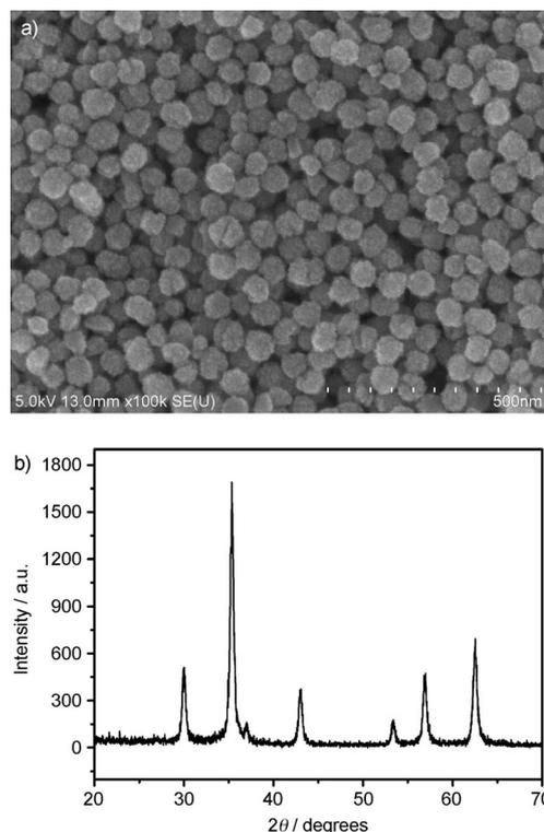
Figure 1. a) Typical SEM image and b) XRD results of the catalyst.
