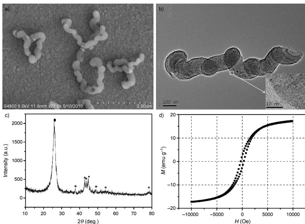
Figure 2. a) Typical SEM image, b) TEM image, c) XRD (● = graphite, ■ =  $\alpha$ -Fe, and \* =  $\text{Fe}_3\text{C}$ ), and d) magnetization curve of the HCNTs. Inset: HR-TEM image of the HCNTs.
