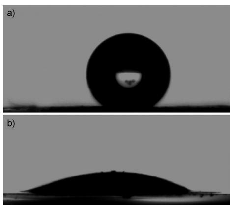
Figure 3. Contact angles of a) HCNTs and b) PAH-functionalized HCNTs.
