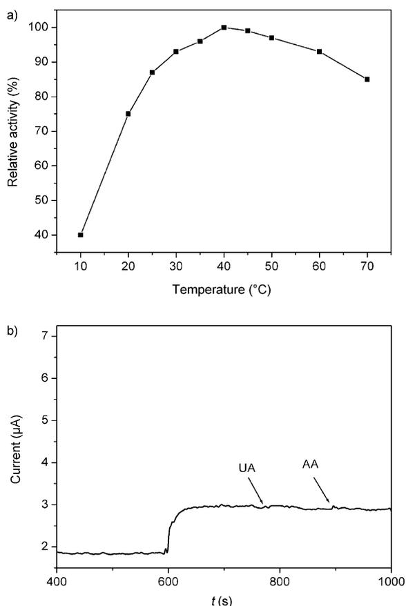
Figure 8. a) Effect of temperature on the electrocatalytic response of HCNTs to  $\text{H}_2\text{O}_2$  reduction. b) Effect of interfering species on the sensor response with  $10 \mu\text{M}$  of  $\text{H}_2\text{O}_2$  in  $0.1 \text{ M}$  PBS (pH 7.0).
