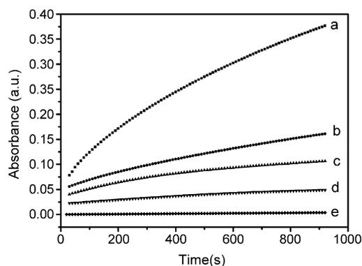
Figure 6. Time-dependent absorbance changes at  $652 \text{ nm}$  in the presence of HCNTs (a), m-HCNTs (b), l-HCNTs (c), MWCNTs (d), and the remaining solution after removal of the HCNTs, which were incubated in the pH 4.0 reaction buffer for 10 min at  $40^\circ\text{C}$  (e).
