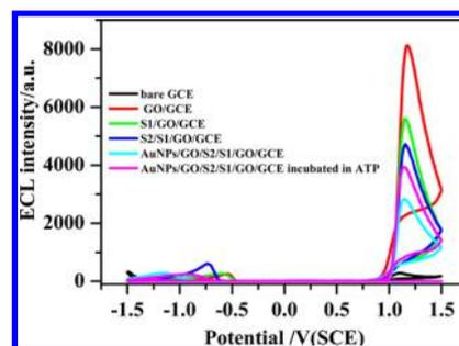
Figure 4. ECL profiles of different modified electrodes in  $66 \mu\text{M}$   $\text{Ru}(\text{bpy})_3^{2+}$  and  $0.1 \text{ mol L}^{-1}$  PBS. Potential scan rate,  $100 \text{ mV s}^{-1}$ ; pH, 7.4.
