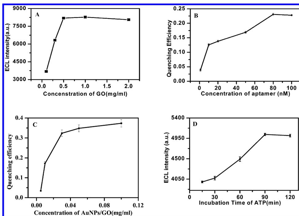
**Figure 6.** (A) Effects of GO concentration on ECL signals. (B) Effect of aptamer concentration on ECL signals. (C) Quenching effect of AuNPs/GO on ECL signals. (D) Effect of the incubation time in 50 pM ATP on ECL intensity.
