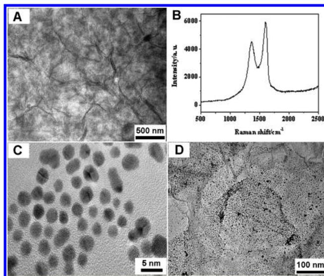
**Figure 3.** (A) SEM image of GO, (B) Raman spectrum of GO, (C) TEM image of AuNPs, and (D) SEM image of AuNPs/GO.
