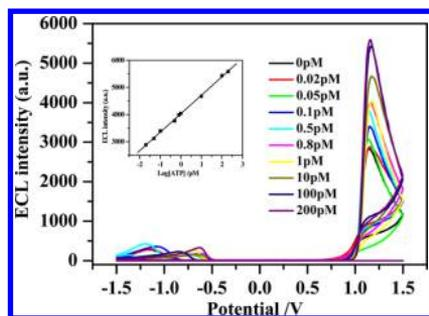
**Figure 7.** ECL curves of the aptasensor incubated in 0.02, 0.05, 0.1, 0.5, 0.8, 1, 10, 100, and 200 pM ATP. The inset is the calibration curve of ATP.
