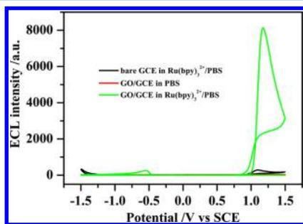
**Figure 1.** ECL curves of the GO/GCE in 0.1 mol L<sup>-1</sup> PBS and the bare GCE and the GO/GCE in 0.1 mol L<sup>-1</sup> PBS containing 66 μM Ru(bpy)<sub>3</sub><sup>2+</sup>. Potential scan rate, 100 mV s<sup>-1</sup>; pH, 7.4.
