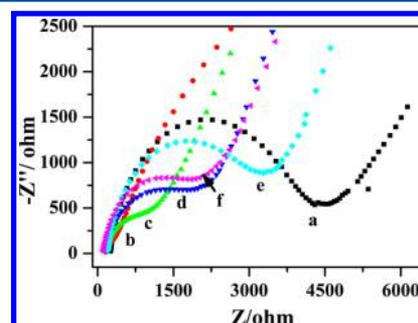
Figure 5. Electrochemical impedance spectroscopy of bare GCE (a), GO/GCE (b), S1/GO/GCE (c), S2/S1/GO/GCE (d), AuNPs/GO/S2/S1/GO/GCE (e), and AuNPs/GO/S2/S1/GO/GCE incubated in  $1 \text{ pM}$  ATP (f).
