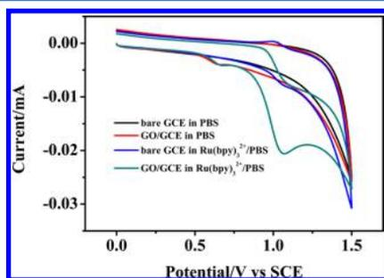
**Figure 2.** Cyclic voltammograms of bare GCE and GO/GCE in Ru(bpy)<sub>3</sub><sup>2+</sup>/PBS. PBS, 0.1 mol L<sup>-1</sup>; Ru(bpy)<sub>3</sub><sup>2+</sup>, 66 μM; pH, 7.4; scan rate, 100 mV s<sup>-1</sup>.
