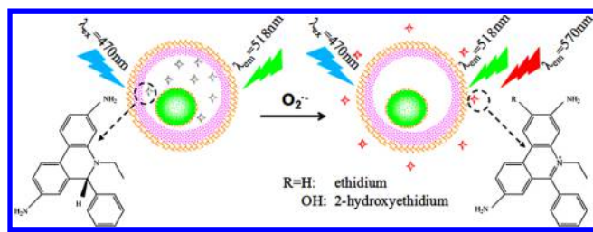
Scheme 1. Ratiometric Fluorescent Biosensing and Imaging of O_2^{\bullet-} Based on the FMH NPs-HE Sensor
