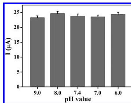
**Figure 8.** Photocurrent responses of the ATP aptasensor after being incubated in Tris-HCl buffer with varied pH from 9.0 to 6.0. The error bars show the standard deviation of five replicate determinations.
