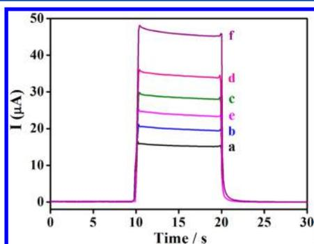
**Figure 5.** Photocurrent responses of (a) the ITO/TiO<sub>2</sub>/Au electrode, (b) after pDNA and MCH immobilization, (c) after anchoring CdS:Mn-NH<sub>2</sub> nanocrystals, (d) after further anchoring Ru(bpy)<sub>2</sub>(dcbpy)<sup>2+</sup> dyes, (e) after cDNA hybridization, and (f) after incubation with 20 μL of 100 nM ATP.
