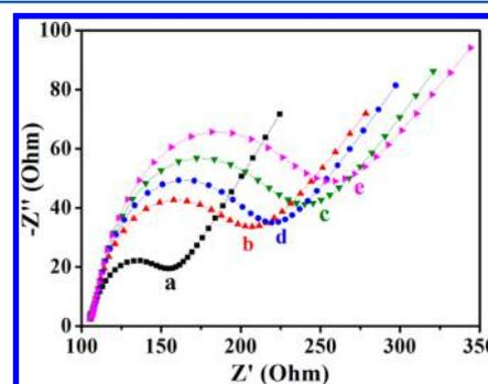
**Figure 4.** EIS of (a) the ITO/ $\text{TiO}_2$ /Au electrode, (b) after pDNA and MCH immobilization, (c) after anchoring CdS:Mn- $\text{NH}_2$  nanocrystals, (d) after further anchoring  $\text{Ru}(\text{bpy})_2(\text{dcbpy})^{2+}$  dyes, and (e) after cDNA hybridization.
