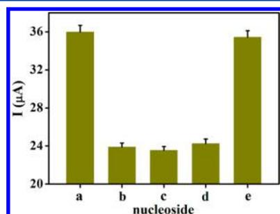
**Figure 7.** Photocurrent responses of the aptasensor to (a) 100 pM ATP, 1 nM (b) CTP, (c) GTP, (d) UTP, and (e) all of their mixture. The error bars show the standard deviation of five replicate determinations.
