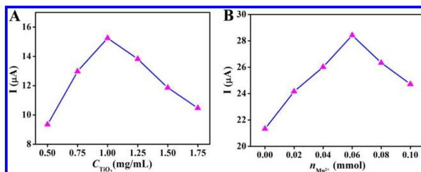
**Figure 3.** Effect of (A)  $\text{TiO}_2$  concentration on photocurrent intensity of ITO/ $\text{TiO}_2$ /Au electrode and (B) mole amount of  $\text{Mn}^{2+}$  on photocurrent intensity of ITO/ $\text{TiO}_2$ /Au/pDNA/MCH/CdS:Mn electrode.
