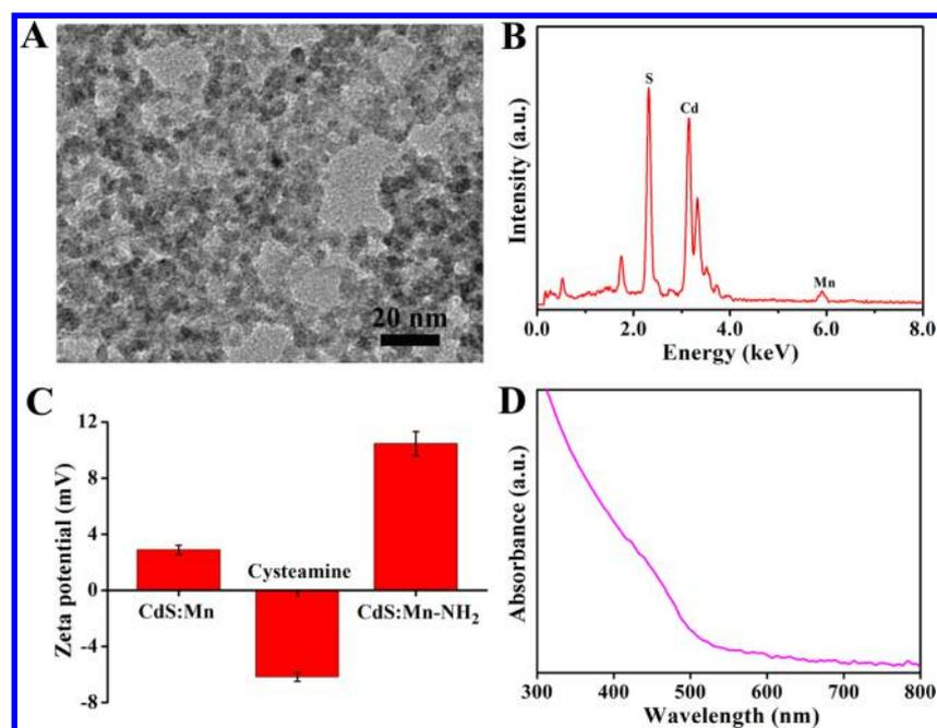
**Figure 1.** (A) TEM image and (B) EDX spectrum of the bare CdS:Mn nanocrystals; (C)  $\zeta$  potentials of the bare CdS:Mn, cysteamine, and CdS:Mn-NH<sub>2</sub>; (D) UV-vis absorption spectrum of the CdS:Mn-NH<sub>2</sub> nanocrystals.
