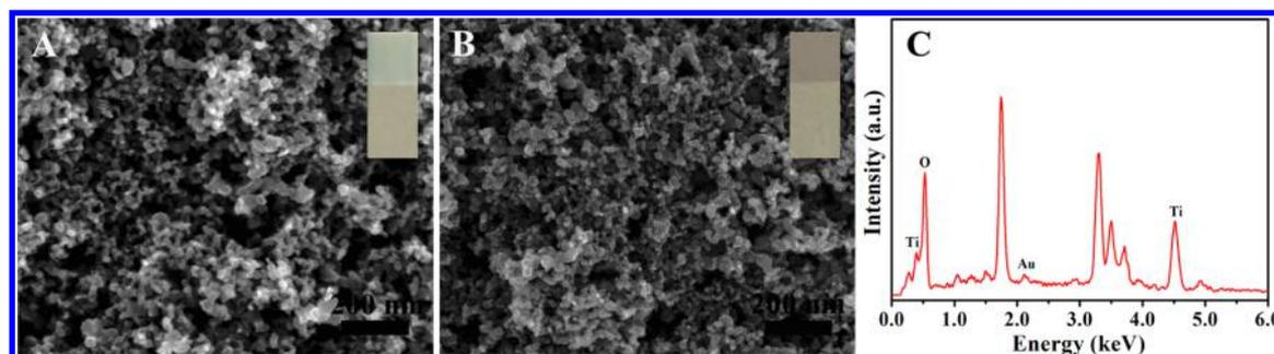
**Figure 2.** Typical SEM images of the (A) ITO/TiO<sub>2</sub> and (B) ITO/TiO<sub>2</sub>/Au electrodes; (C) EDX spectrum of the ITO/TiO<sub>2</sub>/Au electrode. Insets in parts A and B: photograph images of the corresponding electrodes.
