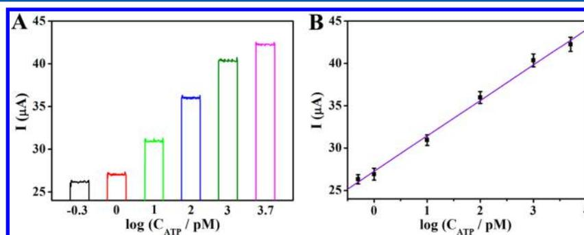
**Figure 6.** (A) Photocurrent response and (B) calibration curve of the aptasensor for the detection of different concentrations of ATP from 0.5 pM to 5 nM. The error bars show the standard deviation of five replicate determinations.
