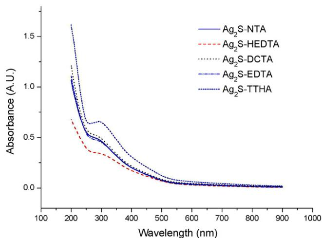
Fig. 1. Absorption spectra of aminopolycarboxyl-modified  $\text{Ag}_2\text{S}$  nanoparticles.
