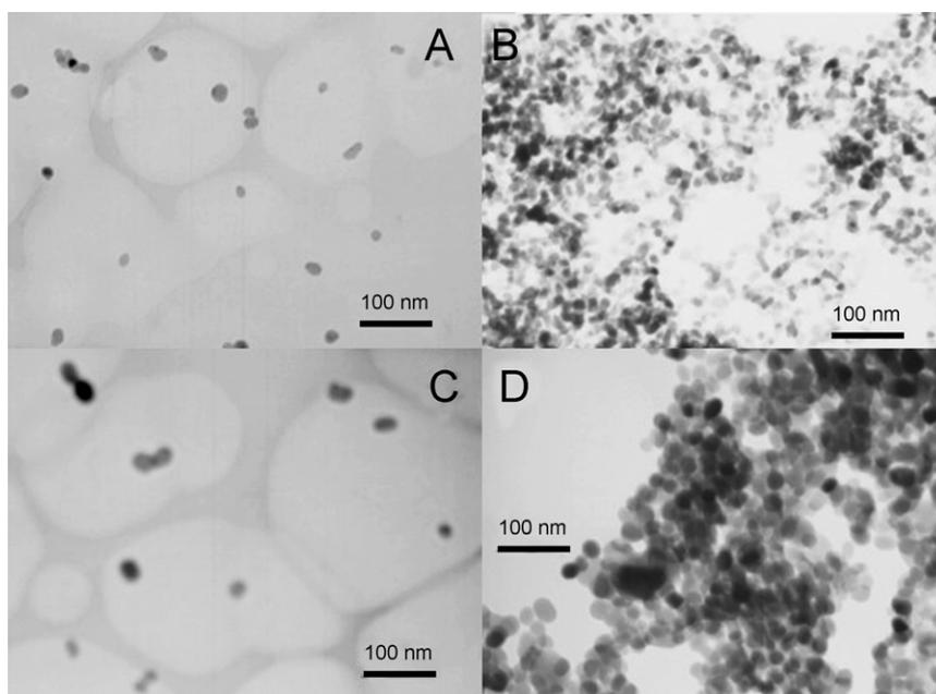
Fig. 4. TEM images:  $\text{Ag}_2\text{S}$  nanoparticles modified with NTA in the absence (A) and presence (B) of BSA;  $\text{Ag}_2\text{S}$  nanoparticles modified with EDTA in the absence (C) and presence (D) of BSA.
