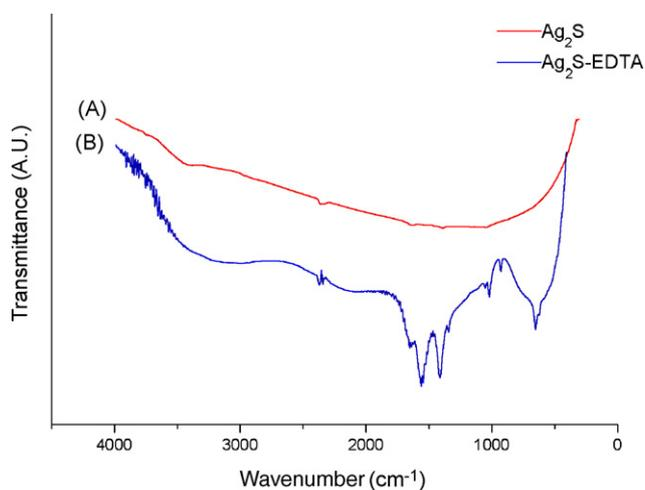
Fig. 2. Representative FTIR spectra of  $\text{Ag}_2\text{S}$  nanoparticles modified with and without EDTA. (A)  $\text{Ag}_2\text{S}$  nanoparticles; (B)  $\text{Ag}_2\text{S}$  nanoparticles modified with EDTA.
