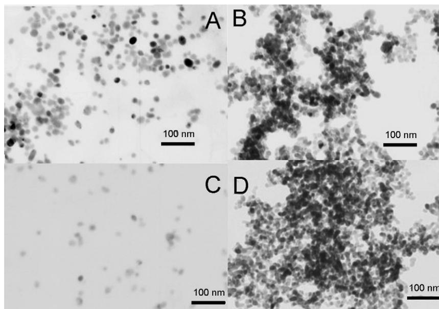
Fig. 3. TEM images:  $\text{Ag}_2\text{S}$  nanoparticles modified with TTHA in the absence (A) and presence (B) of BSA;  $\text{Ag}_2\text{S}$  nanoparticles modified with DCTA in the absence (C) and presence (D) of BSA.
