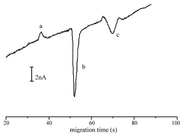
Fig. 4. Electropherogram in glass channel for effective mobilities determination of electroactive analytes. Peak a, vacancy zone of DHBA; peak b, AP zone; peak c, sampling zone corresponding to EOF. Experimental parameters: sample 30 mM MES/His + 0.7 mM AP; running buffer 20 mM MES/His + 0.1 mM DHBA pH 6.00; sampling voltage 800 V; sampling time 2 s; separation voltage 1000 V; detection potential  $+1.2$  V.
