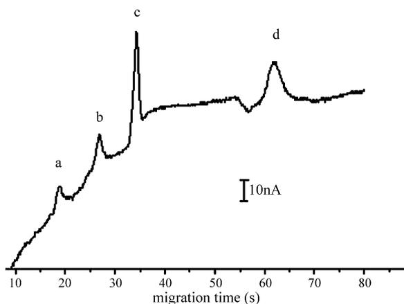
Fig. 3. Electropherogram for anodic EOF measurement in glass channel. Peaks a and b, coions in the sample; peak c, vacancy zone of DHBA; peak d, sampling zone corresponding to EOF. Experimental parameters: sample 12 mM borate + 0.2 mM CTAB pH 9.19; running buffer 15 mM borate + 0.3 mM CTAB + 0.1 mM DHBA pH 9.19; sampling voltage  $-800$  V; sampling time 2 s; separation voltage  $-1000$  V; detection potential  $+1.2$  V.
