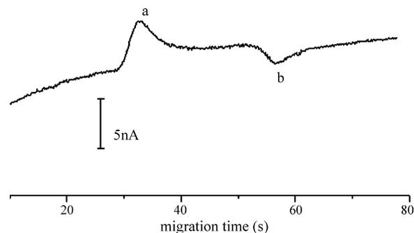
Fig. 2. Electropherogram in hybrid PDMS/glass channel for cathodic EOF measurement. Peak a, vacancy zone of DHBA; peak b, sampling zone corresponding to EOF. Experimental parameters: sample 30 mM PBS; running buffer 20 mM PBS + 0.1 mM DHBA pH 6.95; sampling voltage 800 V; sampling time 2 s; separation voltage 1000 V; detection potential +1.2 V.
