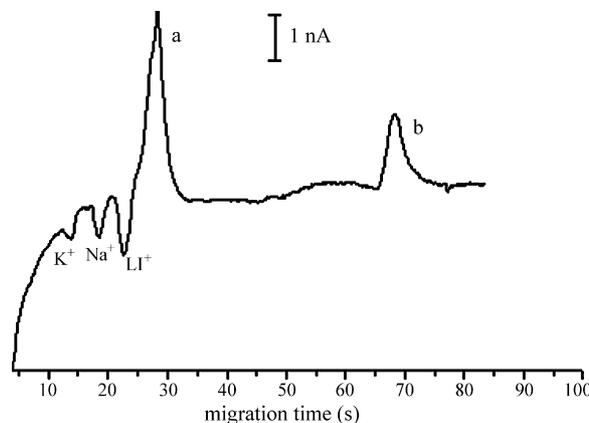
Fig. 5. Electropherogram in glass channel of  $200 \mu\text{M}$   $\text{K}^+$ ,  $\text{Na}^+$  and  $\text{Li}^+$ . Peak a, vacancy zone of DHBA; peak b, sampling zone corresponding to EOF. Experimental parameters: running buffer 20 mM MES/His + 0.1 mM DHBA pH 6.00; sampling voltage 800 V; sampling time 2 s; separation voltage 1000 V; detection potential  $+1.2$  V.
