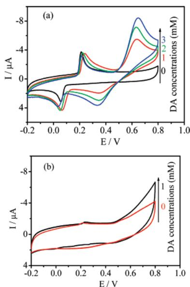
**Figure 8.** Cyclic voltammograms of (a) Au/PPy/Ag-modified GCE and (b) PPy/Ag-modified GCE in the absence and presence of different concentrations of DA at a scan rate 100  $\text{mV/s}$ . Synthetic conditions:  $[\text{AgNO}_3]/[\text{pyrrole}]$  0.7; PVP concentration 2%; reaction time 48 h; room temperature.
