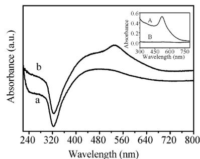
**Figure 6.** UV-vis spectra of (a) PPY/Ag and (b) Au/PPY/Ag. The insets show the UV-vis spectra of the as-prepared colloidal gold solution (A) and the gold solution after reaction with PPY and centrifugation (B). Synthetic conditions:  $[\text{AgNO}_3]/[\text{pyrrole}]$  0.7; PVP concentration 2%; reaction time 48 h; room temperature.
