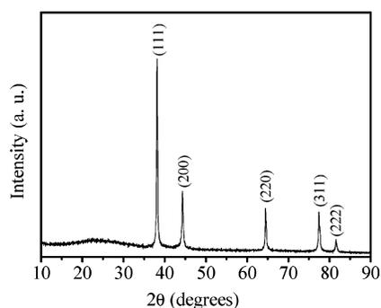
**Figure 3.** XRD pattern of PPy-coated Ag nanocomposite. Synthetic conditions: [AgNO<sub>3</sub>]/[pyrrole] 0.7; PVP concentration 2%; reaction time 48 h; room temperature.
