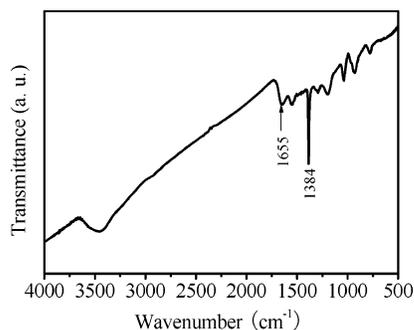
**Figure 4.** FTIR spectrum of PPY-coated Ag nanocomposite. Synthetic conditions:  $[\text{AgNO}_3]/[\text{pyrrole}]$  0.7; PVP concentration 2%; reaction time 48 h; room temperature.
