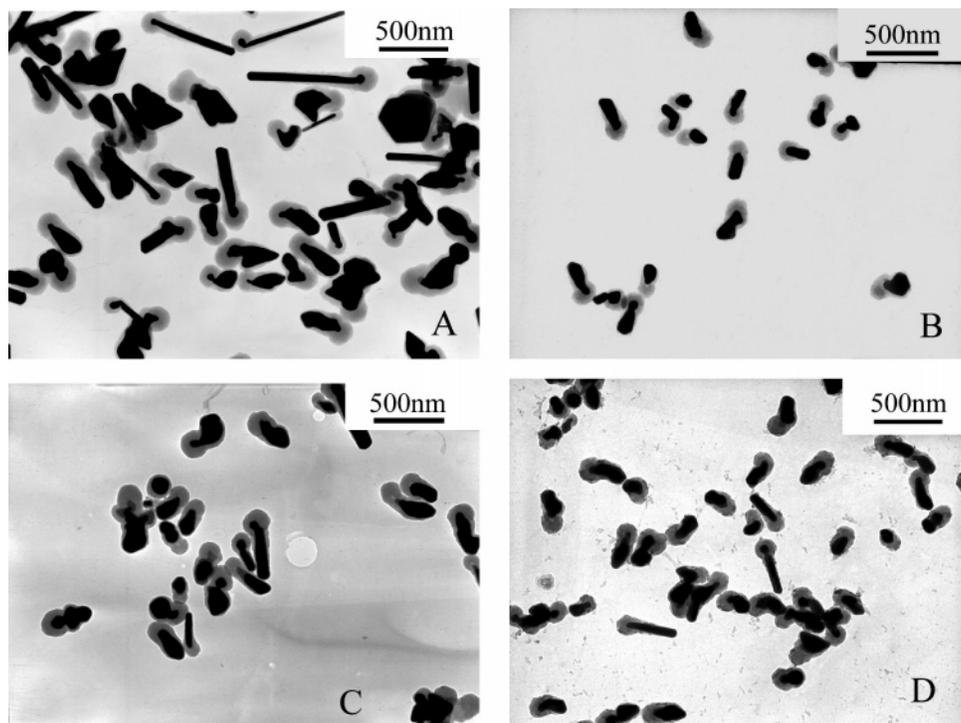
**Figure 2.** TEM images of PPy-coated Ag composites prepared at different molar ratios of AgNO<sub>3</sub> to pyrrole monomer: (A) 1, (B) 0.7, (C) 0.5, and (D) 0.25. Synthetic conditions: PVP concentration 2%; reaction time 48 h; room temperature.
