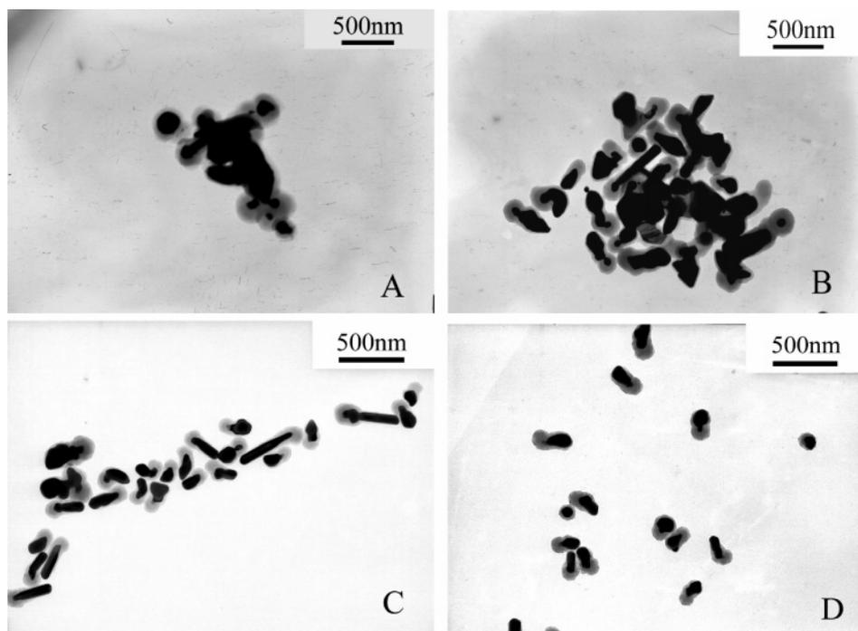
**Figure 1.** TEM images of PPy-coated Ag composites prepared at different PVP concentrations: (A) 0.2%, (B) 0.5%, (C) 1%, and (D) 2%. Synthetic conditions: pyrrole 1 mmol; AgNO<sub>3</sub> 0.12 g; reaction time 48 h; room temperature.
