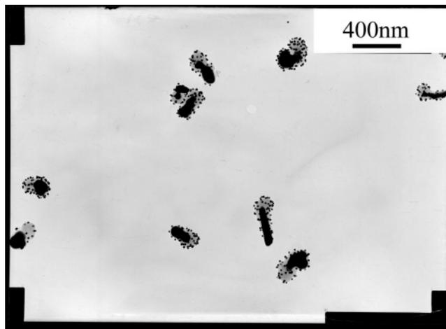
**Figure 5.** TEM image of three-layered Au-modified PPY-coated Ag nanocomposite. Synthetic conditions:  $[\text{AgNO}_3]/[\text{pyrrole}]$  0.7; PVP concentration 2%; reaction time 48 h; room temperature.
