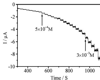
**Figure 9.** Typical steady-state response of Au/PPy/Ag-modified GCE on successive injection of different concentrations of DA into pH 1  $\text{H}_2\text{SO}_4$  solution while stirring with an applied potential of 635  $\text{mV}$ . Synthetic conditions:  $[\text{AgNO}_3]/[\text{pyrrole}]$  0.7; PVP concentration 2%; reaction time 48 h; room temperature.
