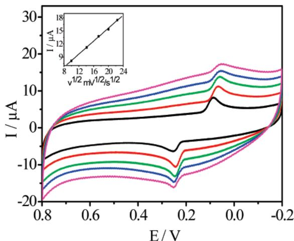
**Figure 7.** Cyclic voltammograms of Au/PPy/Ag-modified GCE measured in pH 1  $\text{H}_2\text{SO}_4$  solution at different scanning rates: from inner to outer 100, 200, 300, 400, 500  $\text{mV s}^{-1}$ . The inset shows the calibration plot between the anodic peak current and the square root of the scanning rate. Synthetic conditions:  $[\text{AgNO}_3]/[\text{pyrrole}]$  0.7; PVP concentration 2%; reaction time 48 h; room temperature.
