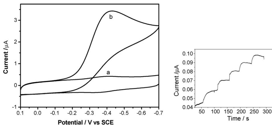
Fig. 7. Cyclic voltammograms of Hb-Gel/GCE in the absence of  $\text{H}_2\text{O}_2$  (a) and in the presence of  $\text{H}_2\text{O}_2$  0.6 mM (b) in 0.1 M pH 7.0 PBS at scan rate of 100 mV/s. Side curve is current–time plot with Hb/gelatine/GC upon the addition of 0.05 mM  $\text{H}_2\text{O}_2$  in the 0.1 M phosphate buffer solution at pH 7.0 at  $-0.38$  V.
