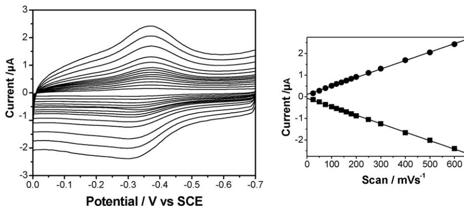
Fig. 4. Typical cyclic voltammograms of Hb-Gel/GCE at different scan rates (from inner to outer): 25, 50, 75, 100, 120, 140, 160, 180, 200, 250, 300, 400, 500, and 600  $\text{mV s}^{-1}$  in the 0.1 M phosphate buffer (pH 7.0). Side figure shows the peak current dependence on the scan rate,  $\nu$ .
