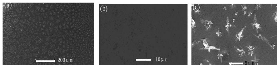
Fig. 1. SEM images of (a) gelatine, (b) Hb and (c) cross-linked Hb + gelatine films.
