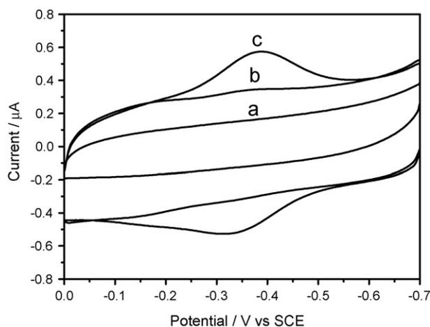
Fig. 3. Cyclic voltammograms of bare GC electrode (a), Gel/GC electrode (b), and Hb-Gel/GC electrode (c) in 0.1 M pH 7.0 PBS.
