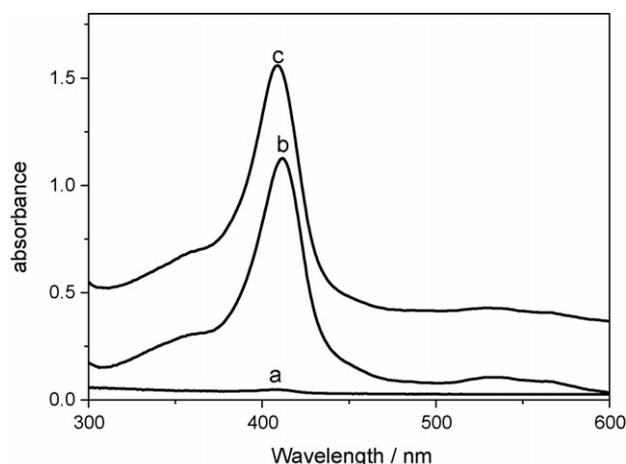
Fig. 2. UV-vis spectra curves: (a) gelatine, (b) Hb, (c) cross-linked Hb + gelatine.
