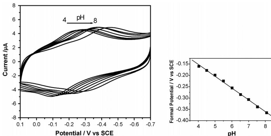
Fig. 6. Cyclic voltammograms of Hb-Gel/GCE in  $0.1$  M PBS with various pH values at scan rate of  $100$   $mV s^{-1}$ . Side figure shows effect of pH on formal potential.
