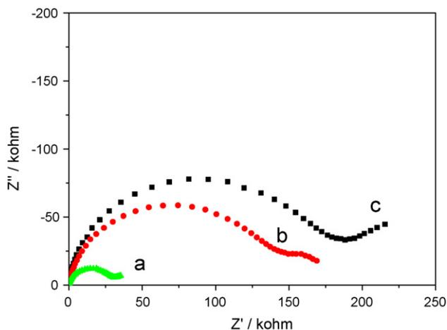
Fig. 5. EIS curves on (a) bare GC electrode, (b) gelatine-modified GC electrode, and (c) Hb/gelatine-modified GC electrode.
