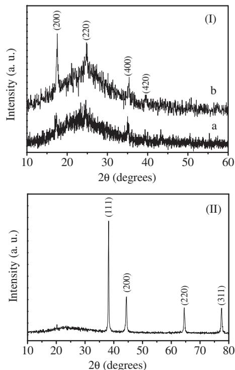
**Figure 5.** XRD patterns of PPy/PB (I) and PPy/Ag (II) composite microtubes. Synthetic conditions of PPy/PB (1) and PPy/Ag (2): (1) pyrrole 105  $\mu$ l, MO 0.05 g, [Py]/[KHCf] 1:2 (a) and 1:10 (b), solvent hydrochloric acid, reaction time 24 h, room temperature; (2) pyrrole 105  $\mu$ l, MO 0.05 g, AgNO<sub>3</sub> 0.24 g, solvent distilled water, UV irradiation time 2 h, room temperature.
