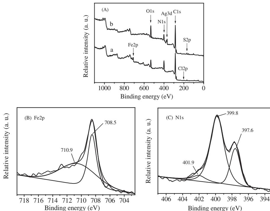
**Figure 7.** (A) XPS spectra of PPy/PB (a) and PPy/Ag (b) composite microtubes; (B) and (C) are the XPS data of the Fe 2p and N 1s regions of the PPy/PB, respectively. Synthetic conditions of PPy/PB (1) and PPy/Ag (2): (1) pyrrole 105  $\mu\text{l}$ , MO 0.05 g, [Py]/[KHCF] 1:10, solvent hydrochloric acid, reaction time 24 h, room temperature; (2) pyrrole 105  $\mu\text{l}$ , MO 0.05 g,  $\text{AgNO}_3$  0.24 g, solvent distilled water, UV irradiation time 2 h, room temperature.
