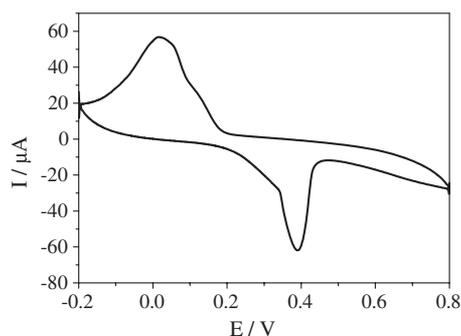
**Figure 9.** Cyclic voltammograms of PPy/Ag composite microtube modified GCE immersed in pH 6 PBS at 100  $\text{mV s}^{-1}$ . Synthetic conditions: pyrrole 105  $\mu\text{l}$ , MO 0.05 g,  $\text{AgNO}_3$  0.24 g, solvent distilled water, UV irradiation time 2 h, room temperature.
