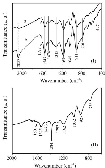
**Figure 6.** FTIR of PPy/PB (I) and PPy/Ag (II) composite microtubes. Synthetic conditions of PPy/PB (1) and PPy/Ag (2): (1) pyrrole 105  $\mu\text{l}$ , MO 0.05 g, [Py]/[KHCF] 1:2 (a) and 1:10 (b), solvent hydrochloric acid, reaction time 24 h, room temperature; (2) pyrrole 105  $\mu\text{l}$ , MO 0.05 g, AgNO<sub>3</sub> 0.24 g, solvent distilled water, UV irradiation time 2 h, room temperature.
