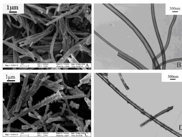
**Figure 1.** SEM and TEM images of PPy/PB composite microtubes synthesized at different concentrations of KHCF. Synthetic conditions: pyrrole 105  $\mu$ l, MO 0.05 g,  $[Py]/[KHCF]$  1:2 (A), (B) and 1:10 (C), (D), solvent hydrochloric acid, reaction time 24 h, room temperature.
