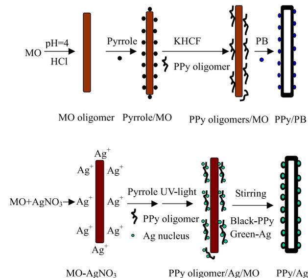
**Scheme 1.** Scheme of the formation of PPy/PB and PPy/Ag composite microtubes.
