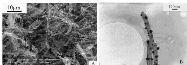
**Figure 2.** SEM (A) and TEM (B) images of PPy/Ag composite microtubes. Synthetic conditions: pyrrole 105  $\mu$ l, MO 0.05 g,  $\text{AgNO}_3$  0.24 g, solvent distilled water, UV irradiation time 2 h, room temperature.
