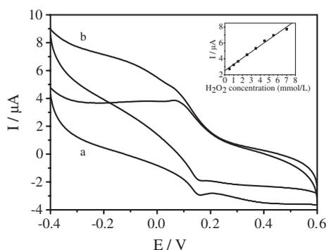
**Figure 8.** Cyclic voltammograms of PPy/PB composite microtube modified GCE immersed in pH 6 PBS without (a) and with (b) 7.0 mM  $\text{H}_2\text{O}_2$  at 100  $\text{mV s}^{-1}$ . The inset shows the changes in the current response under different concentrations of  $\text{H}_2\text{O}_2$ . Synthetic conditions: pyrrole 105  $\mu\text{l}$ , MO 0.05 g, [Py]/[KHCF] 1:10, solvent hydrochloric acid, reaction time 24 h, room temperature.
