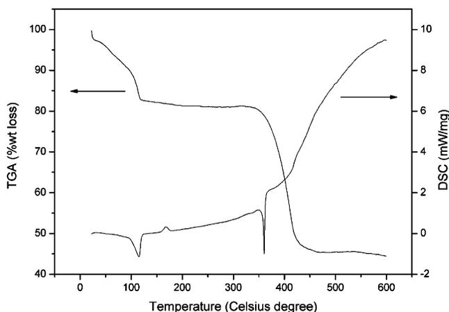
**Figure 3.** Thermal analysis of the  $\text{Znq}_2$  nanorods.
