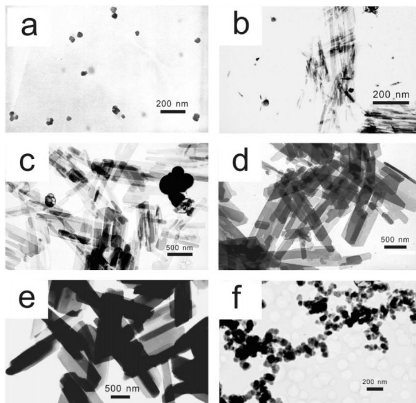
**Figure 5.** TEM images of the products obtained at different reaction conditions: after ultrasound treatment for (a) 1, (b) 3, (c) 6, (d) 12, and (e) 40 min; under electromagnetic stirring instead of ultrasound treatment for (f) 45 min.
