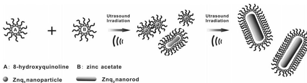
**Figure 6.** Schematic illustration of the formation mechanism of the Znq<sub>2</sub> nanorods.
