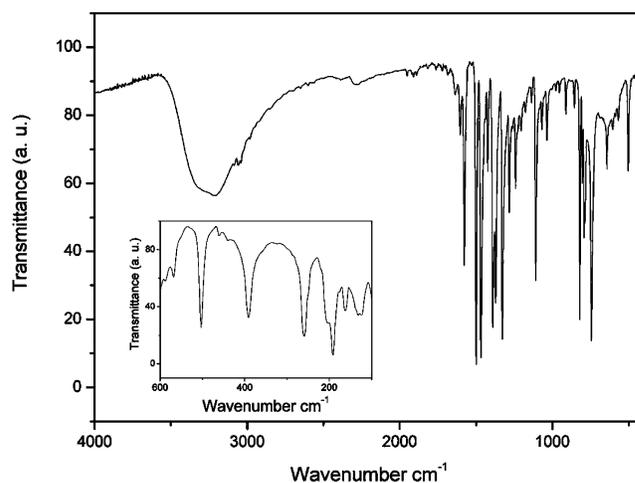
**Figure 2.** IR spectrum of the  $\text{Znq}_2$  nanorods. Inset: Far-IR spectrum.
