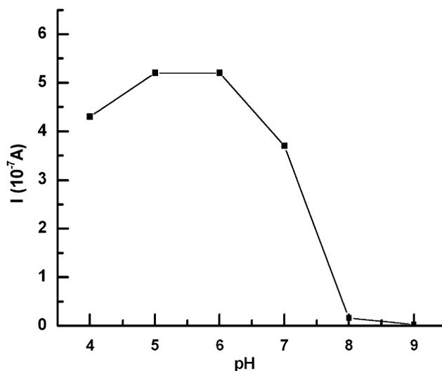
Fig. 5. Influence of pH values of PBS on the response currents of  $10 \mu\text{M H}_2\text{O}_2$  at the HRP–mesoporous PANI film modified electrode.
