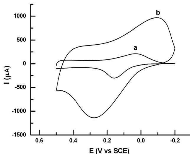
Fig. 3. Cyclic voltammetry of PANI deposited from aqueous solution (a) and LCC template mesoporous PANI (b) in 1 M HClO<sub>4</sub> at the scan rate of 50 mV s<sup>-1</sup>.
