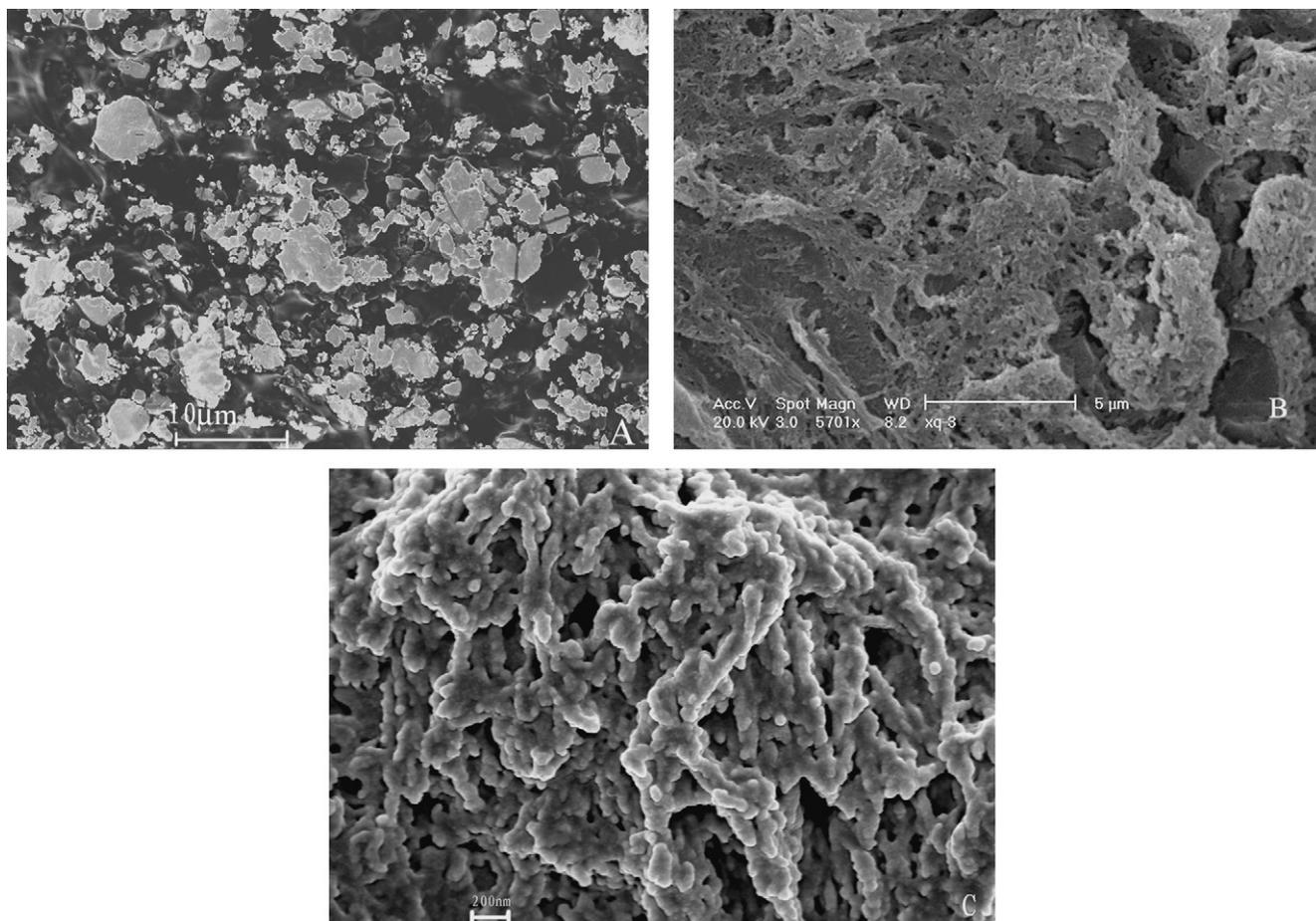
Fig. 1. SEM of PANI deposited from aqueous solution (A) and LCC templated mesoporous PANI (B and C).
