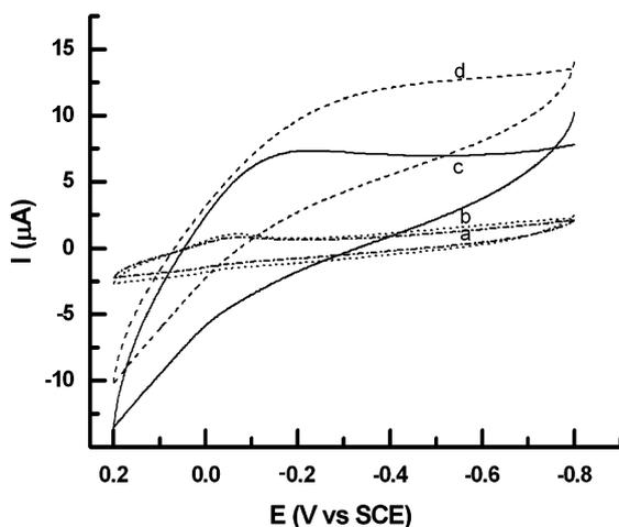
Fig. 4. Cyclic voltammograms of HRP–nonporous PANI film (a and b) and HRP–mesoporous PANI film (c and d) modified electrode in the absence (a and c) and presence of  $2.0 \text{ mmol L}^{-1} \text{ H}_2\text{O}_2$  in 0.1 M PBS 7.0 solution. Scan rate,  $100 \text{ mV s}^{-1}$ .
