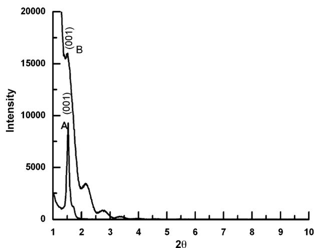
Fig. 2. Low-angle XRD patterns for LCC template aniline electrolyte (A) and mesoporous PANI films (B).
