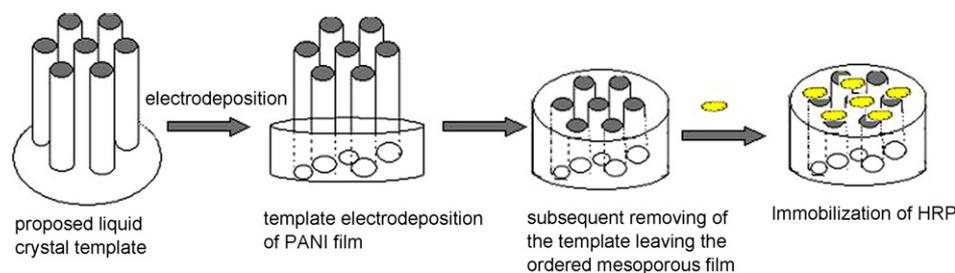
Scheme 1. The formation process of the ordered mesoporous PANI film from the hexagonal lyotropic liquid crystalline (LCC) phase and its application for HRP immobilization.
