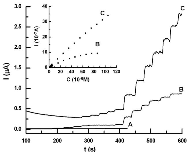
Fig. 6. Typical steady-state response of the biosensor on successive injection of different concentration of  $\text{H}_2\text{O}_2$  into 0.1 M stirring PBS 7.0 solution. Applied potential,  $-100$  mV (A, PANI; B, HRP–nonporous PANI; C, HRP–mesoporous PANI).
