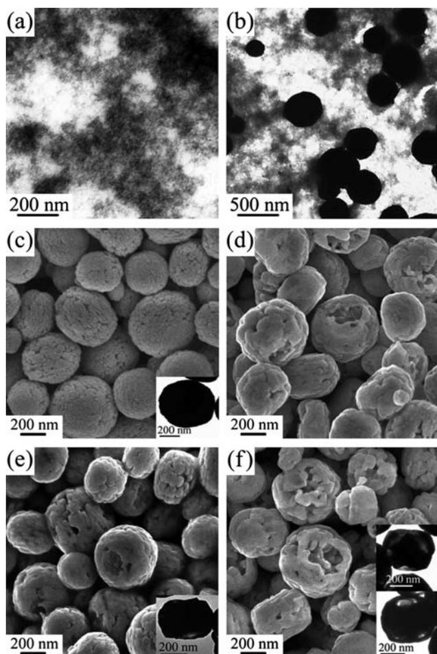
**Fig. 3** TEM and SEM images of  $\text{SmF}_3$  samples obtained by reaction of  $\text{Sm}^{3+}$  with  $\text{NH}_4\text{F}$  in the presence of EDTA (a) without hydrothermal treatment; (b–f) at  $110\text{ }^\circ\text{C}$  for 1, 2, 6, 8 and 12 h. Insets of (c), (e) and (f): TEM images of individual sub-micropumpkins.
