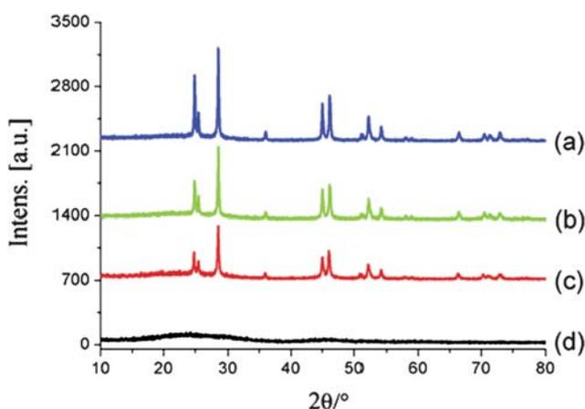
**Fig. 4** XRD patterns for  $\text{SmF}_3$  sub-micropumpkins prepared at  $110\text{ }^\circ\text{C}$  for (a) 12 h, (b) 2 h, (c) 1 h, and (d) without hydrothermal treatment.
