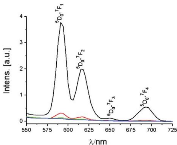
**Fig. 7** Emission spectra of Eu-doped  $\text{SmF}_3$  rattle-structured sub-microcrystals upon the excitation of 325 nm He–Cd laser. Black line:  $\text{Sm}_{0.05}\text{Eu}_{0.95}\text{F}_3$  sub-microcrystals; red line:  $\text{Sm}_{0.25}\text{Eu}_{0.75}\text{F}_3$  sub-microcrystals; green line:  $\text{Sm}_{0.5}\text{Eu}_{0.5}\text{F}_3$  sub-microcrystals; blue line:  $\text{Sm}_{0.75}\text{Eu}_{0.25}\text{F}_3$  sub-microcrystals.
