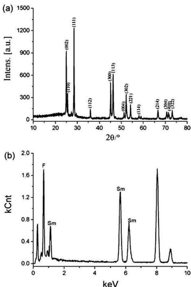
**Fig. 1** (a) XRD pattern and (b) EDX analysis of the product obtained by reaction of  $\text{Sm}^{3+}$  with  $\text{NH}_4\text{F}$  in the presence of EDTA for 16 h.
