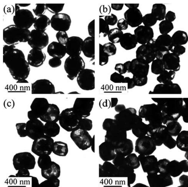
**Fig. 6** TEM images of (a)  $\text{Sm}_{0.75}\text{Eu}_{0.25}\text{F}_3$ , (b)  $\text{Sm}_{0.5}\text{Eu}_{0.5}\text{F}_3$ , (c)  $\text{Sm}_{0.25}\text{Eu}_{0.75}\text{F}_3$  and (d)  $\text{Sm}_{0.05}\text{Eu}_{0.95}\text{F}_3$  sub-microcrystals, which were obtained in the solution with molar ratio of  $\text{Sm}^{3+}$  to  $\text{Eu}^{3+}$  at 3/1, 1/1, 1/3 and 1/19, respectively.
