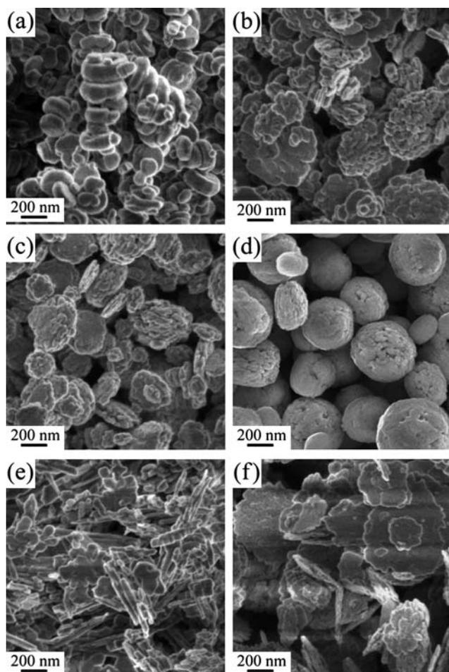
**Fig. 5** SEM images of  $\text{SmF}_3$  samples, obtained by reaction of  $\text{Sm}^{3+}$  with  $\text{NH}_4\text{F}$  at 110 °C for 16 h (a) without EDTA; in the presence of (b) 0.5 mmol EDTA, (c) 1 mmol EDTA, (d) 2.5 mmol EDTA, (e) 1.71 mmol 1,6-hexanediamine and (f) 1.71 mmol ammonium citrate.
