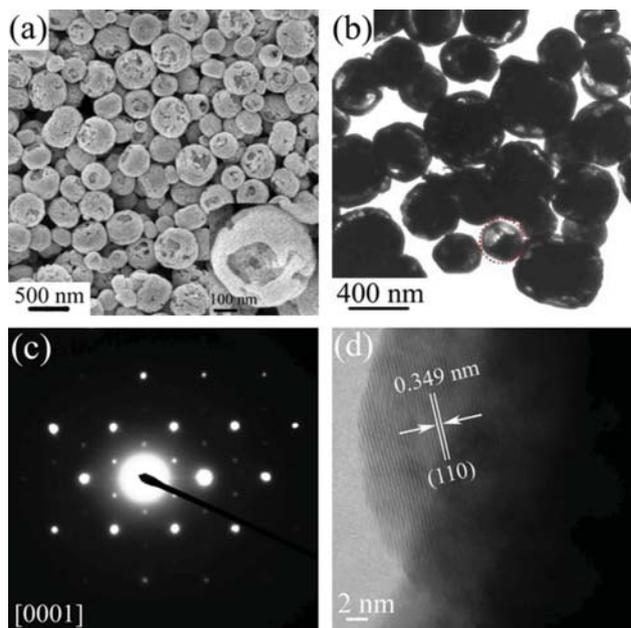
**Fig. 2** (a) SEM and (b) TEM images of  $\text{SmF}_3$  rattle-structured sub-micropumpkins prepared at 110 °C for 16 h; (c) SAED and (d) HRTEM images for an individual rattle-structured sub-micropumpkin. The red circle highlights the semi-hollow sub-micropumpkin.
