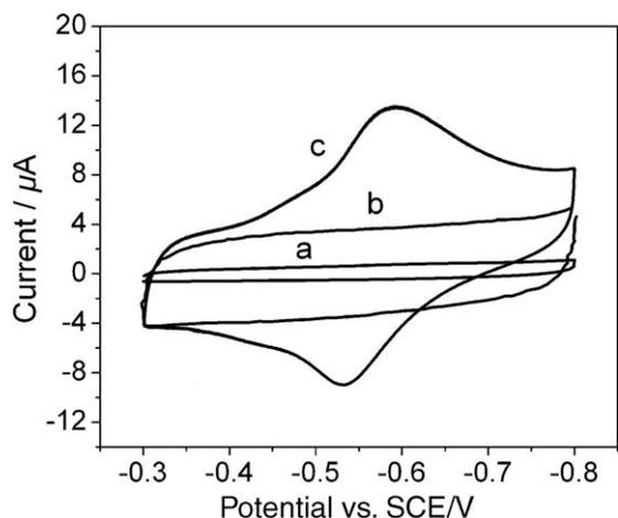
Fig. 3. Cyclic voltammograms of (a) GCE, (b) Ag/Ab<sub>1</sub>/AuNPs/C modified GCE in 0.1 M pH 7.0 PBS, and (c) HRP-Ab<sub>2</sub>/Ag/Ab<sub>1</sub>/AuNPs/C/GCE at in 0.1 M pH 7.0 PBS contained 2.0 mM o-phenylenediamine and 3.0 mM  $\text{H}_2\text{O}_2$ . Scan rate: 100 mV/s.
