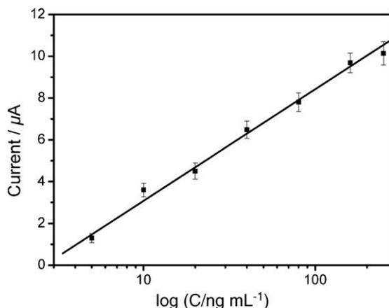
Fig. 5. The resulting calibration curve of HlgG plotted on a semi-log scale.
