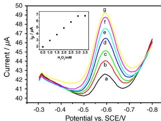
Fig. 4. DPV of HRP-Ab<sub>2</sub>/Ag/Ab<sub>1</sub>/AuNPs/C hybrids modified GCE in 0.1 M pH 7.0 PBS + 2.0 mM o-phenylenediamine with successive addition of 0.5, 1.0, 1.5, 2.0, 2.5, 3.0, and 3.5 mM  $\text{H}_2\text{O}_2$  (from a to g). Inset: the plot of peak current vs.  $\text{H}_2\text{O}_2$  concentration.
